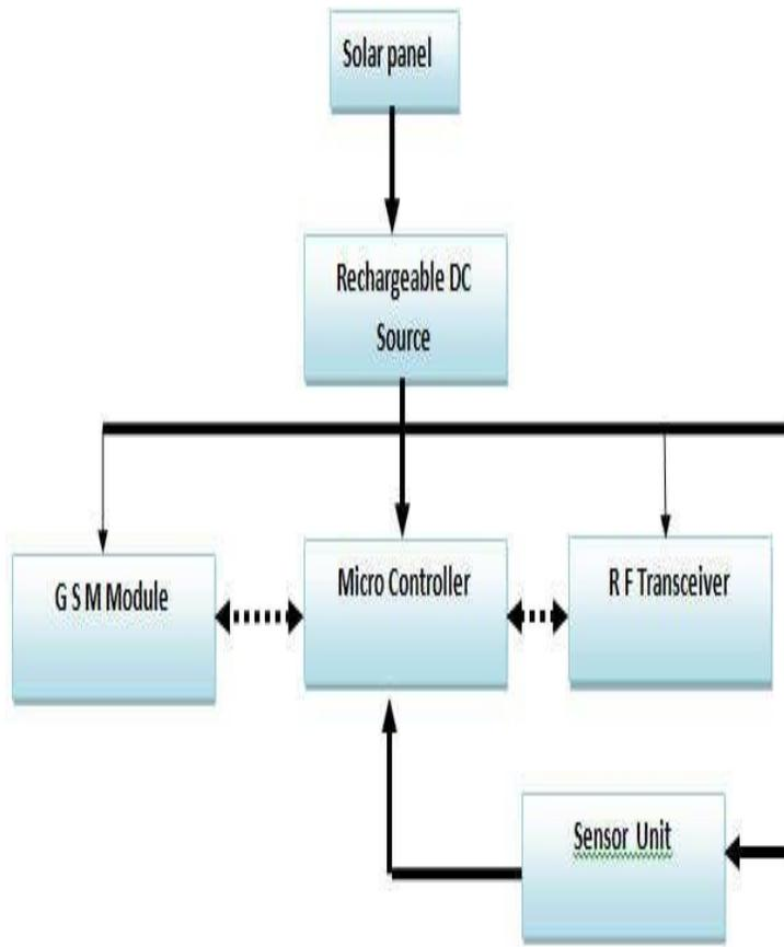
Figure 3.2: System block diagram of the master node
