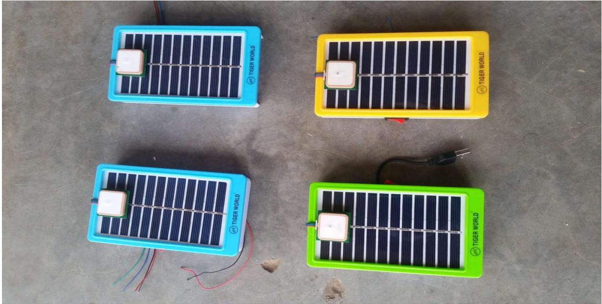
Plate 4.2: Developed Slave Node Prototype
