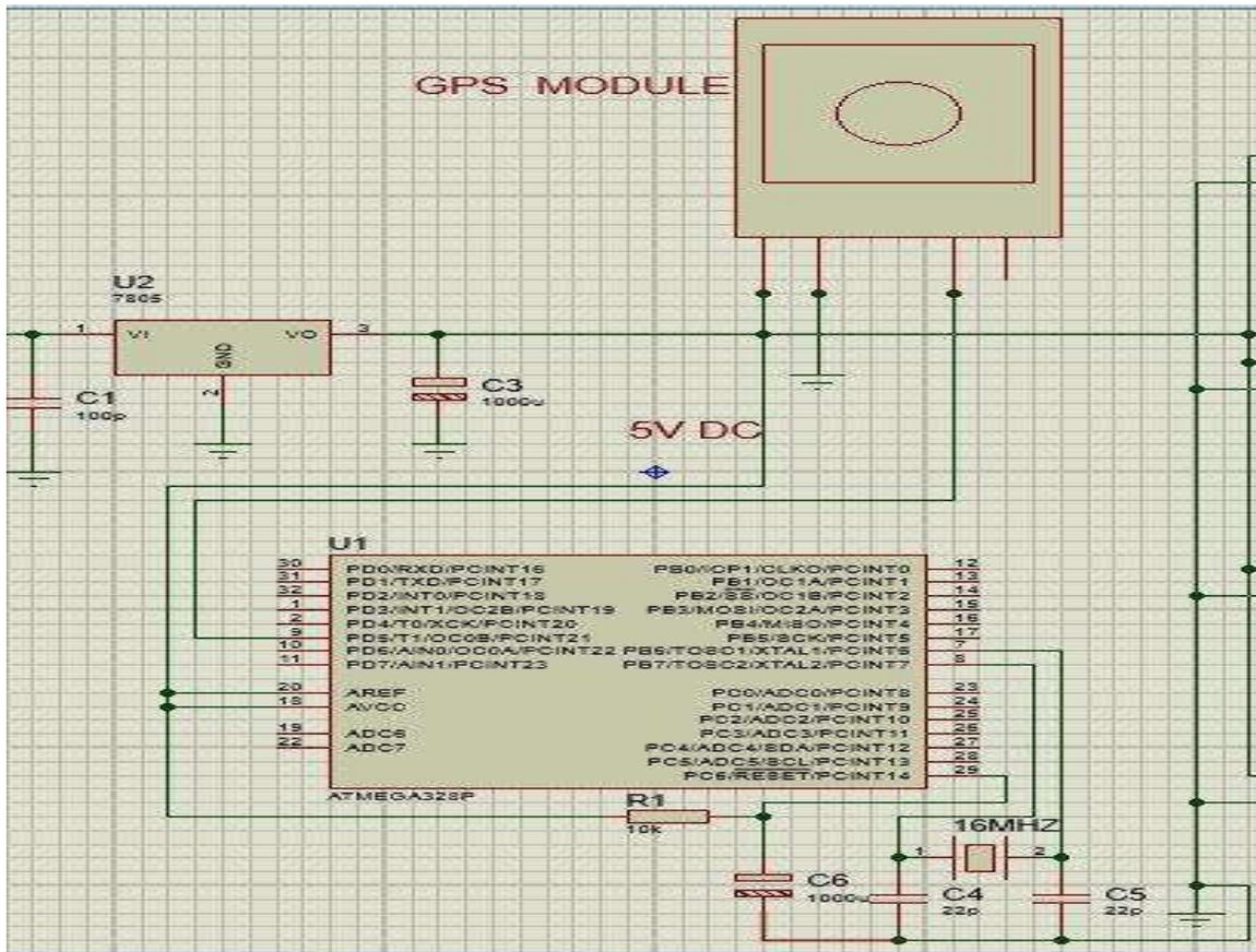
Figure 3.5: GPS Module Interfacing with MCU
