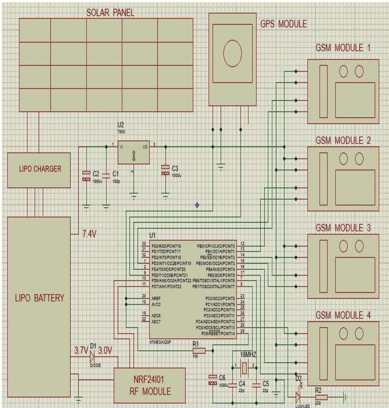
Figure 3.8: Master Node Circuit.
