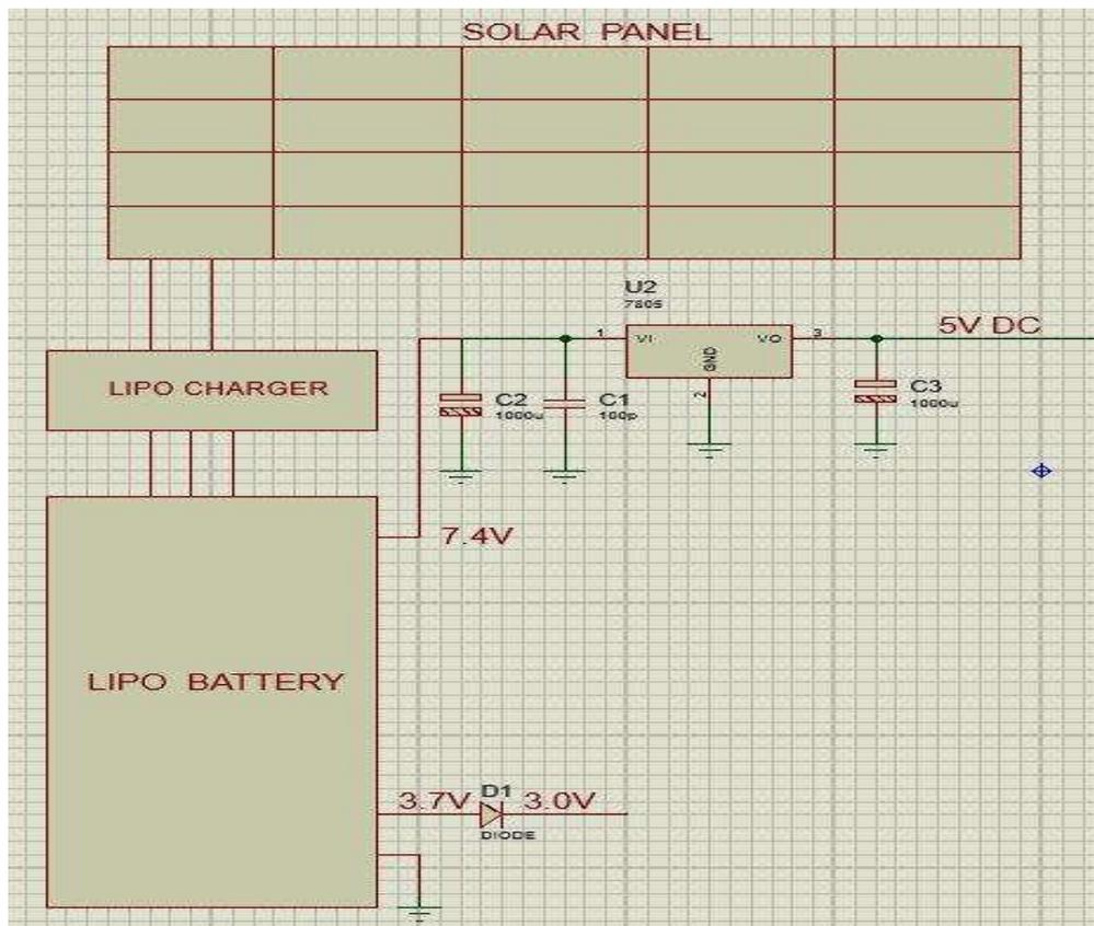
Figure 3.3: Proteus Implementation of the Power Supply Unit
