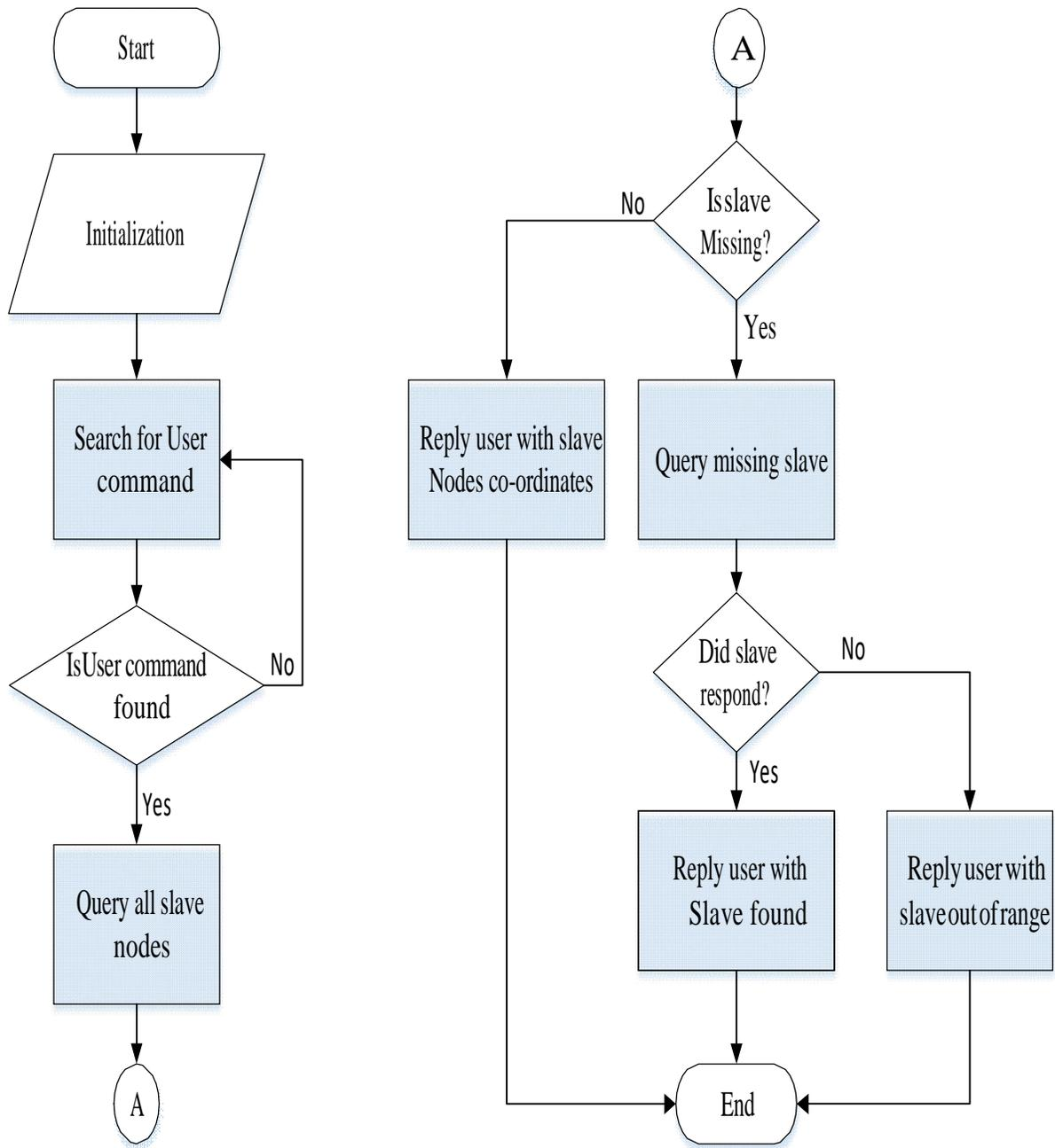
Figure 3.12: Query based Data Transfer between Master node and User node
