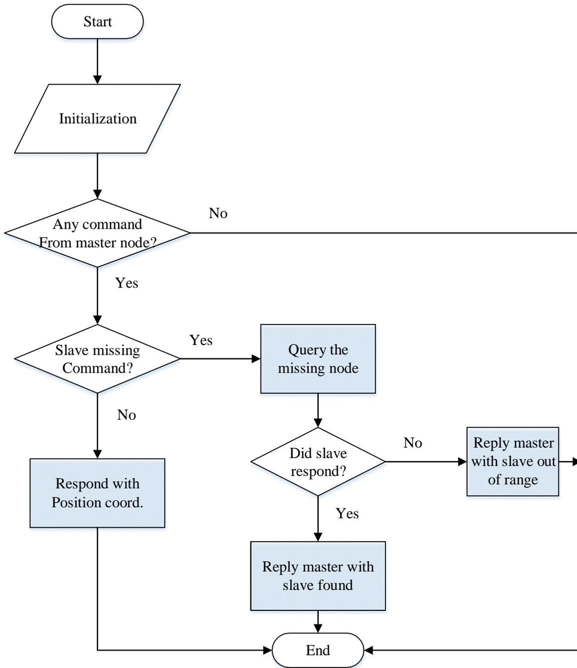
Figure 3.11: Flow Chart for Event based Data Transfer between Master nodes and User node
