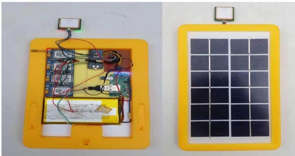
Plate 4.1: Developed Master Node Prototype
