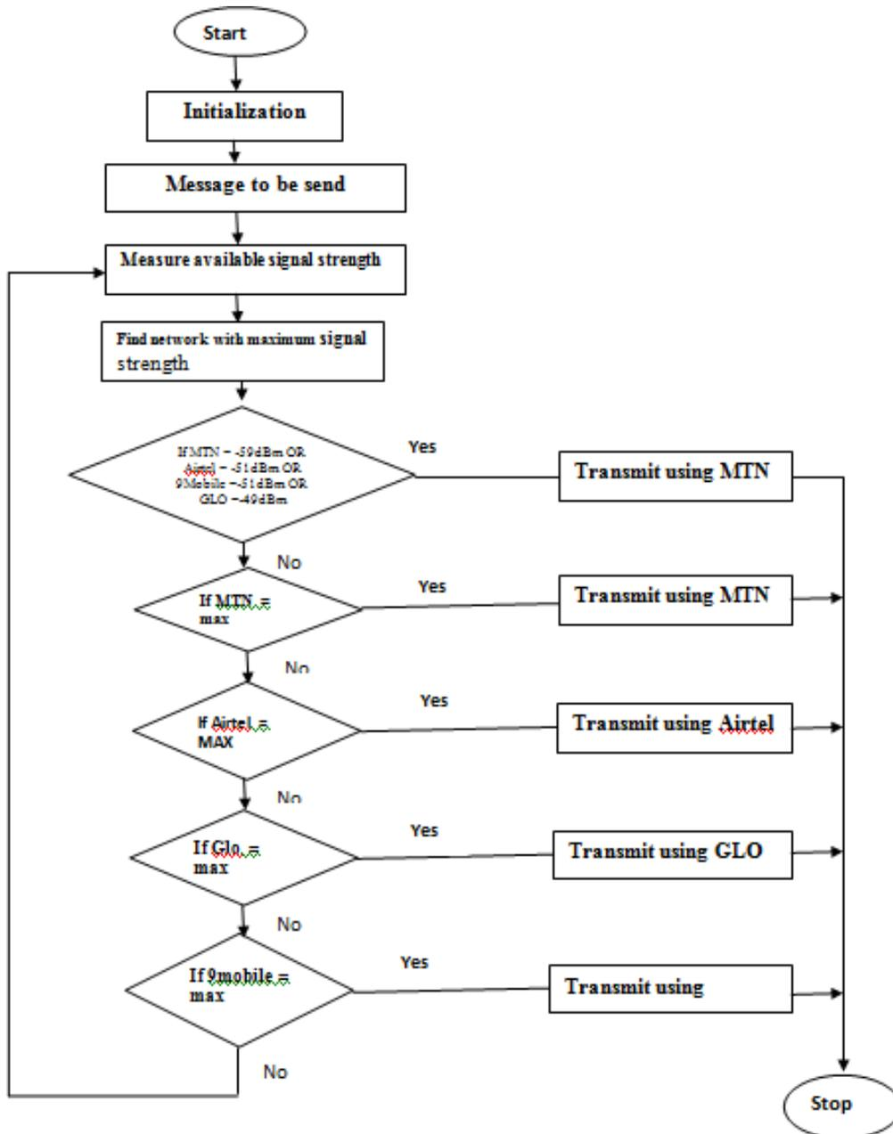
Figure 3.13: Flow chart of Adaptive network selection Scheme
