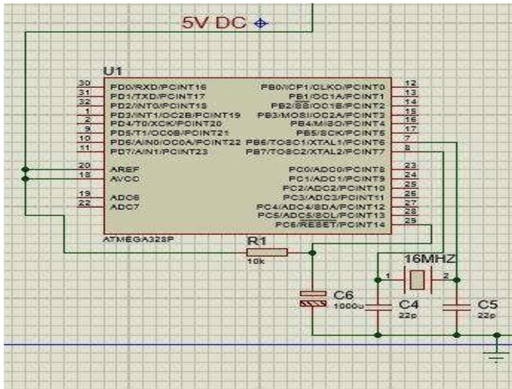
Figure 3.4: Proteus Implementation of MCU Configuration
