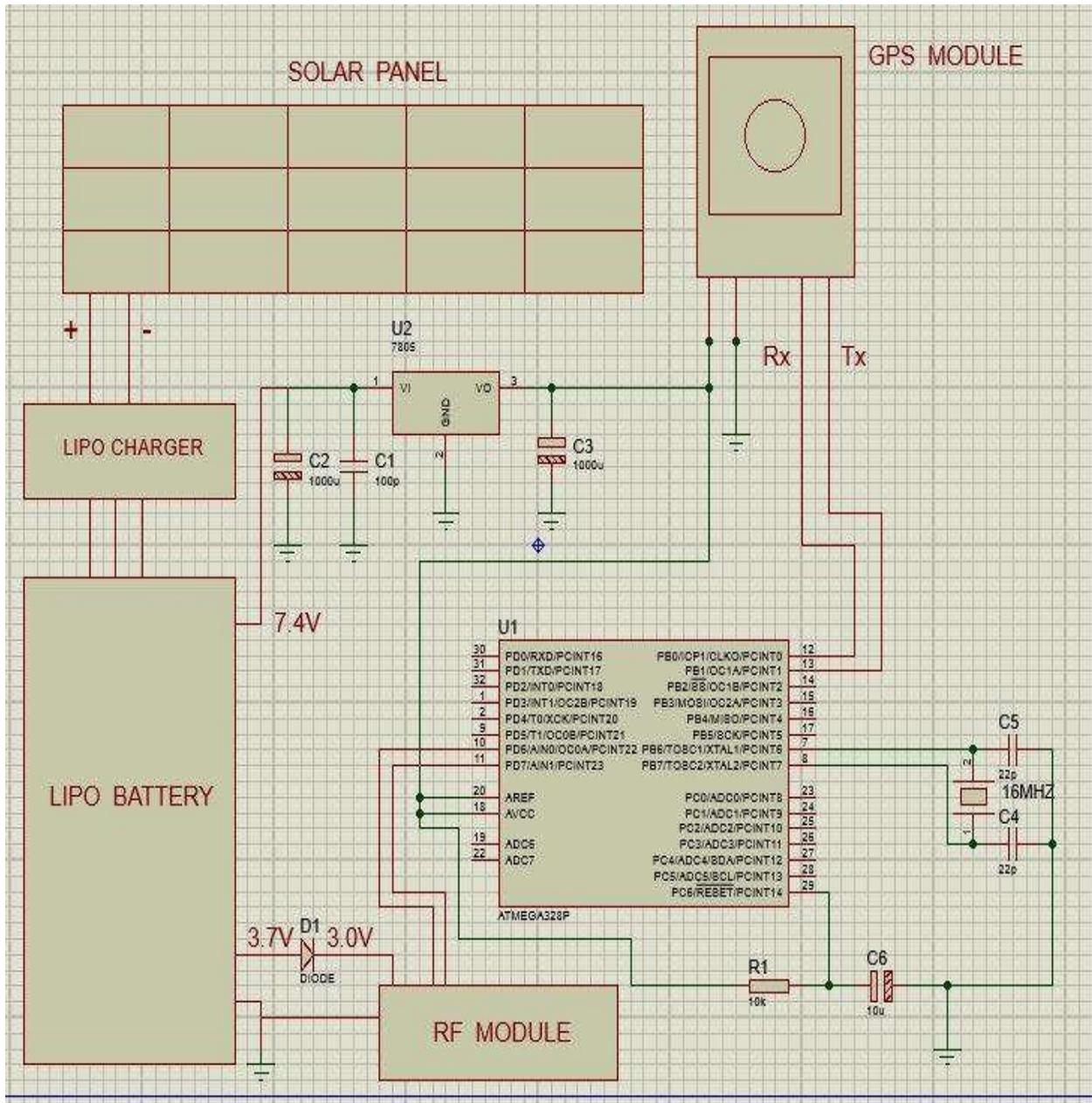
Figure 3.10: Complete Circuitry of the Slave Node.
