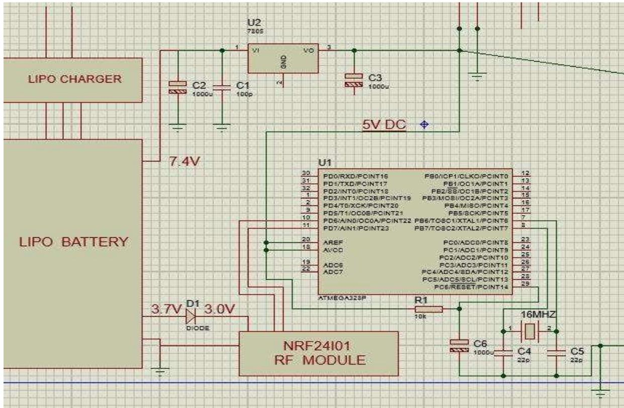
Figure 3.6: Interfacing of RF Module with MCU
