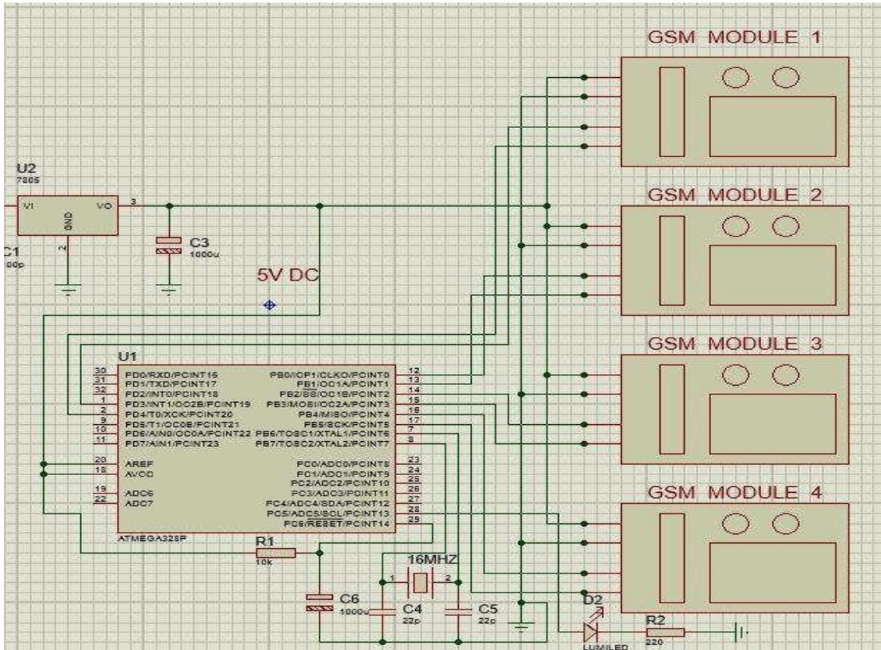
Figure 3.7: GSM Module Interfacing
