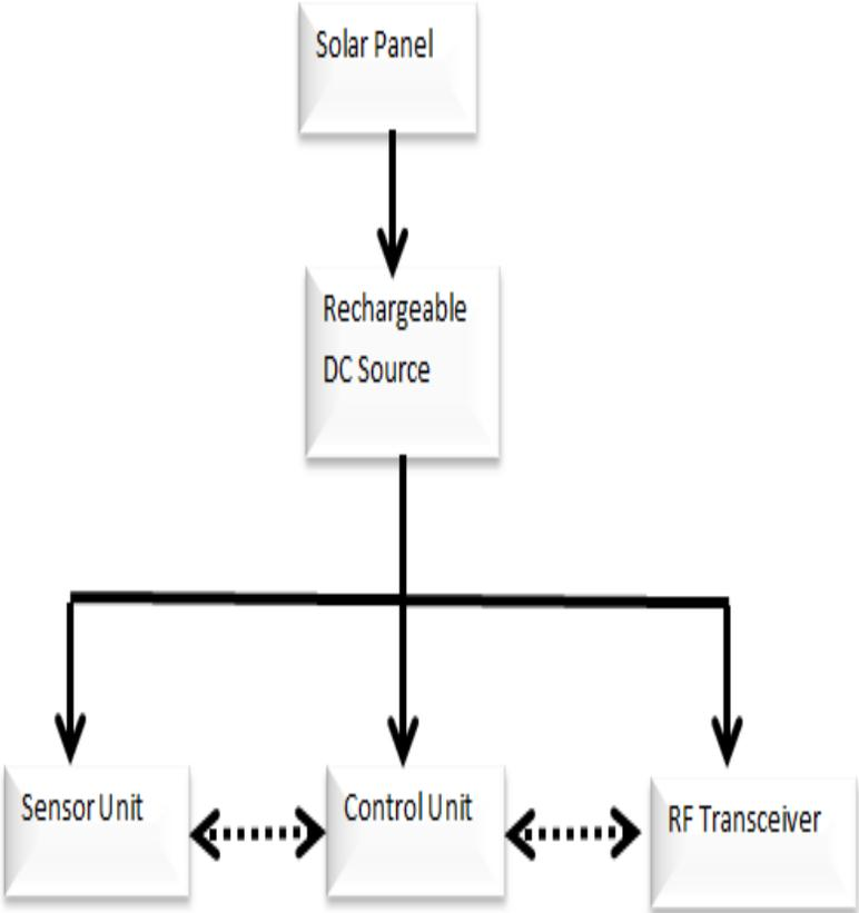
Figure 3.9: Block diagram of slave node
