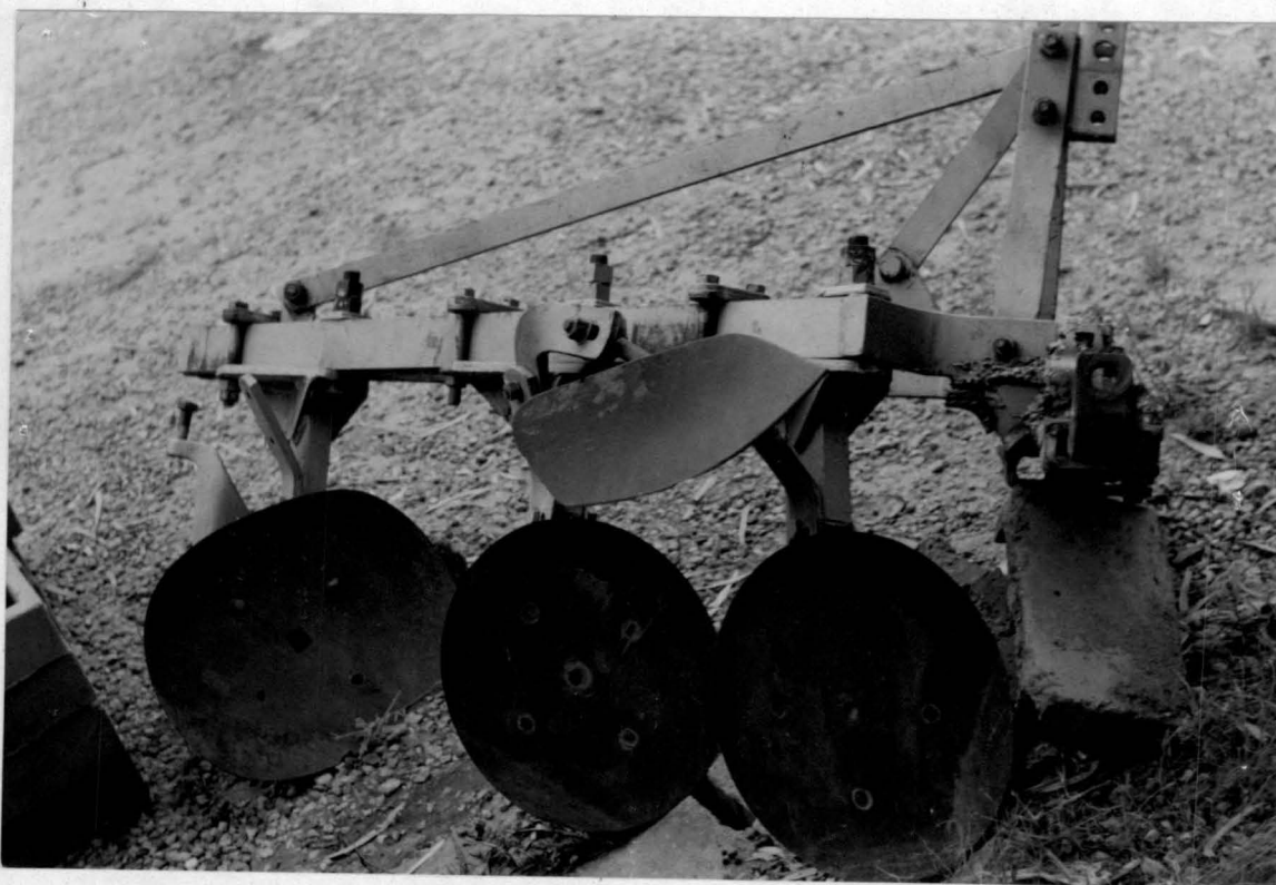
Plate 5: Ford disc plough in poor working condition. Note the Worn out discs, missing furrow wheel and scrapers.
