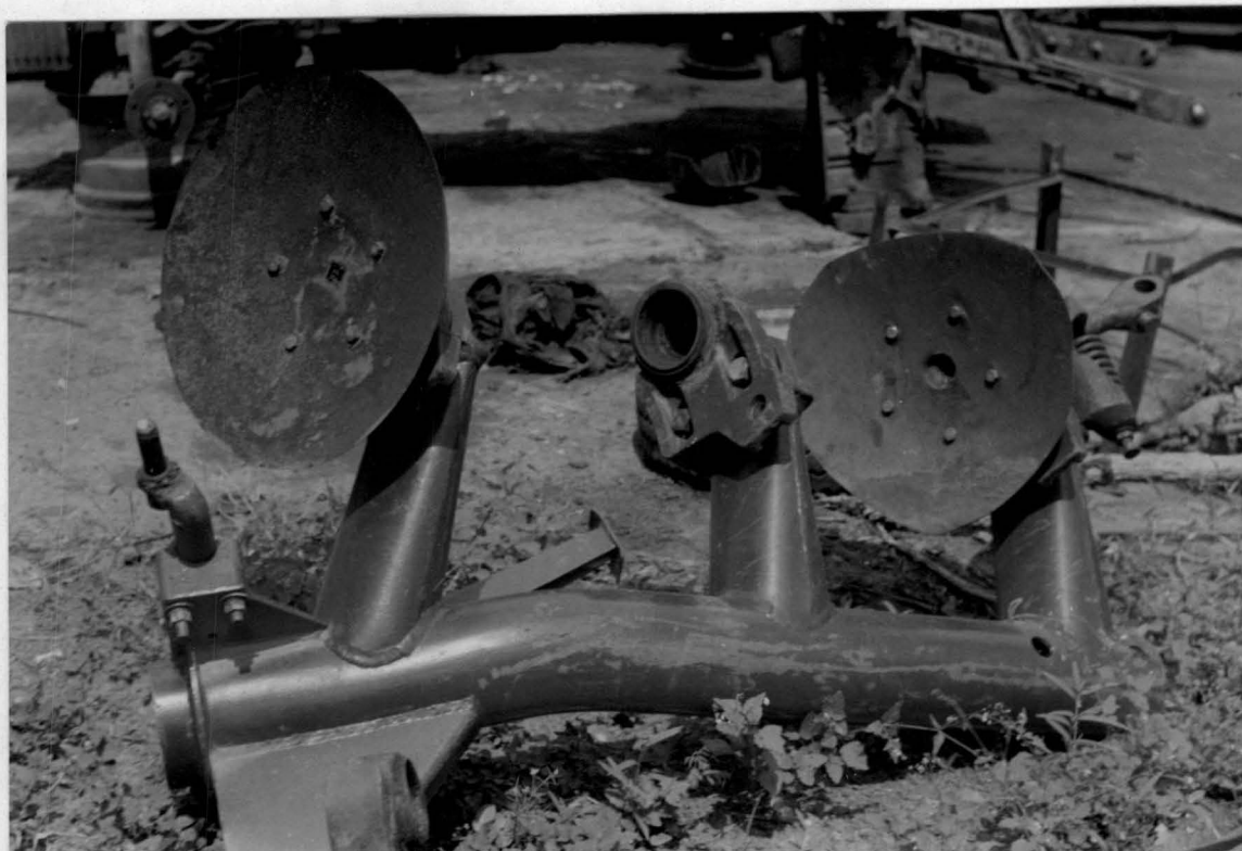
Plate 2: MF disc plough in poor working condition. Note the worn out and missing discs. The furrow wheel is absent
