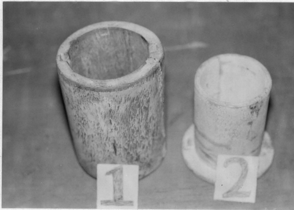
Plate7, The patterns of the sleeve bearing 1 Housing; 2 Bearing.
