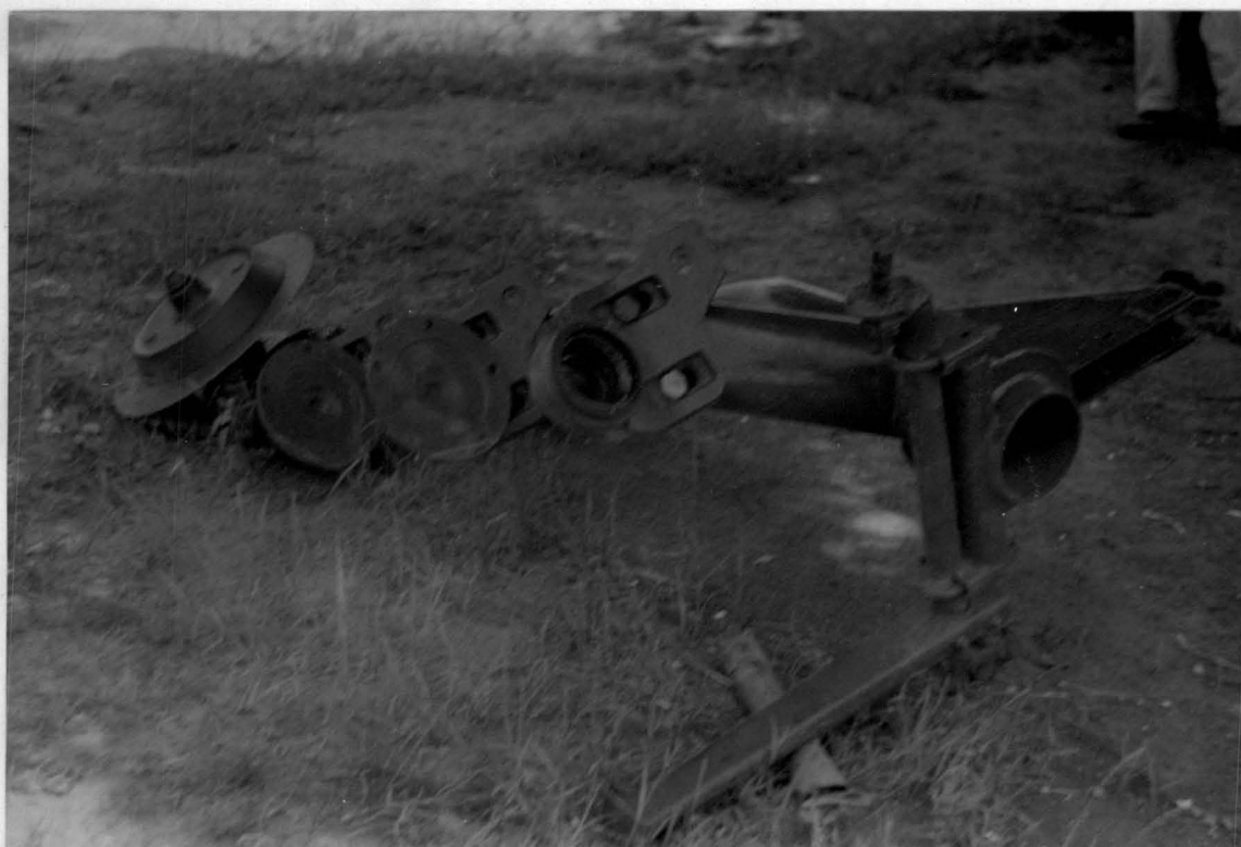
Plate 3: MF disc plough in poor working condition. Note a cap of bearing intact into its hub; a disc mounting and set of discs and scrapers are missing.
