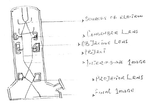
A transmission electron microscope. The beam of electron is emitted from the eletron gun, a heated filament, electrongnets bend of beam.
