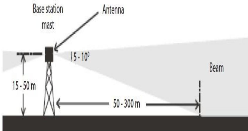
**Figure 2. 2:** Direction of coverage due to a Base Station Antenna
