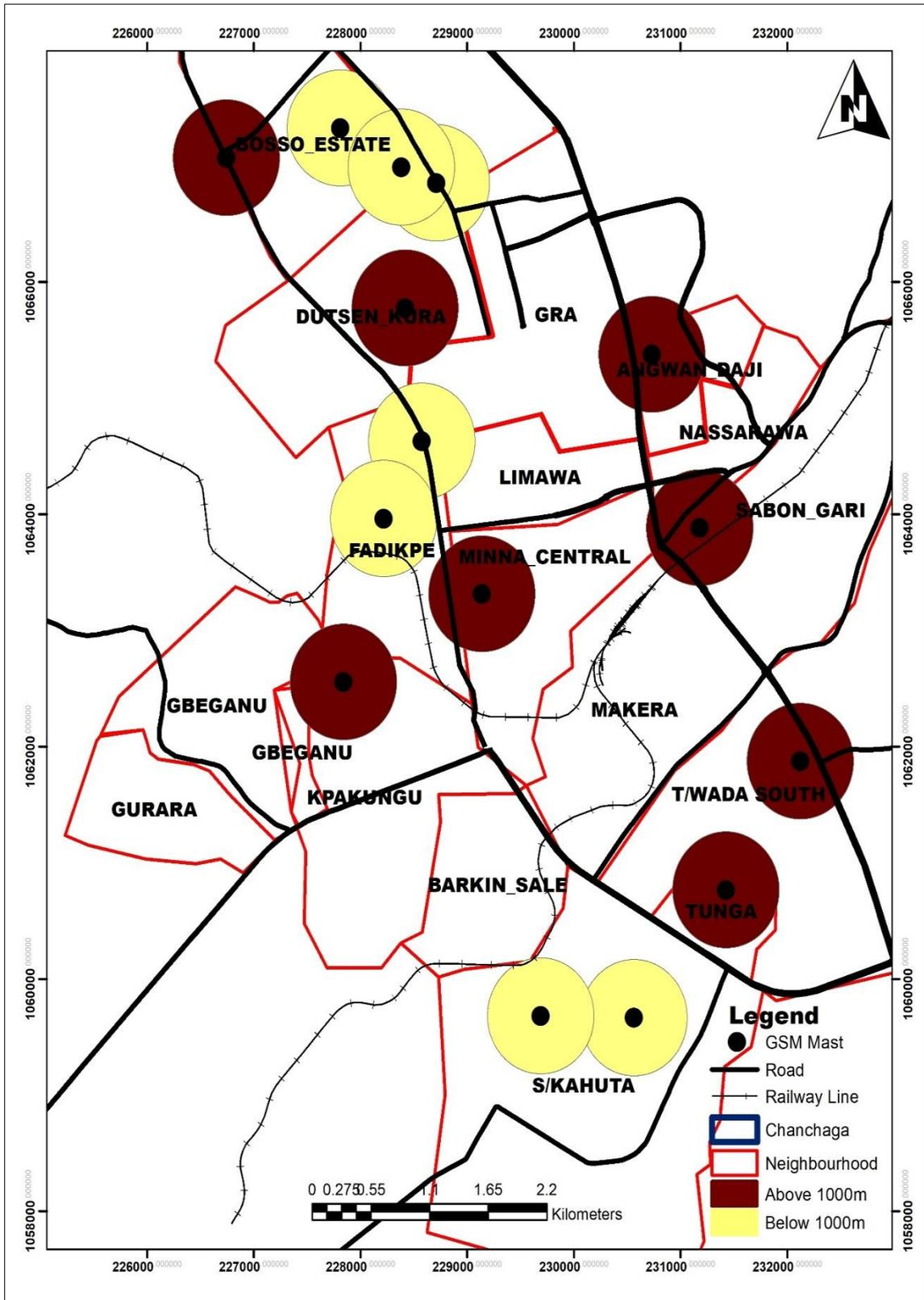
Figure 4.12: 1000m Buffer Analysis of 9Mobile Mast in Minna
