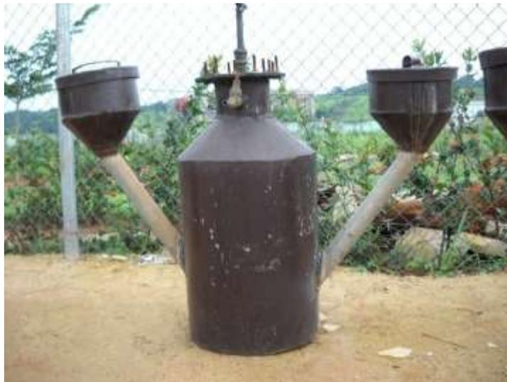
**Plate 3.1: A biodigester**
