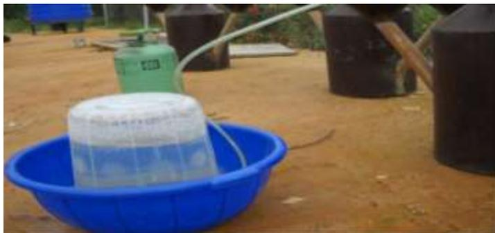
Plate 3.2: Measurement of the volume of biogas produced using displacement method
