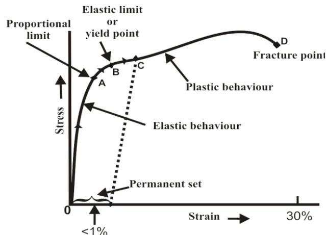
**Figure 2.2: Stress-Strain Diagram of a Ductile Material (Hearn, 2000).**
