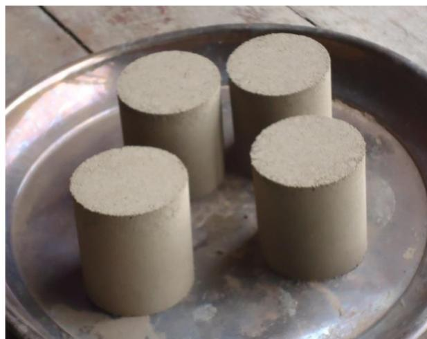
**Plate 3.2: Baked 50 mm  $\times$  50 mm Sand Specimen**
