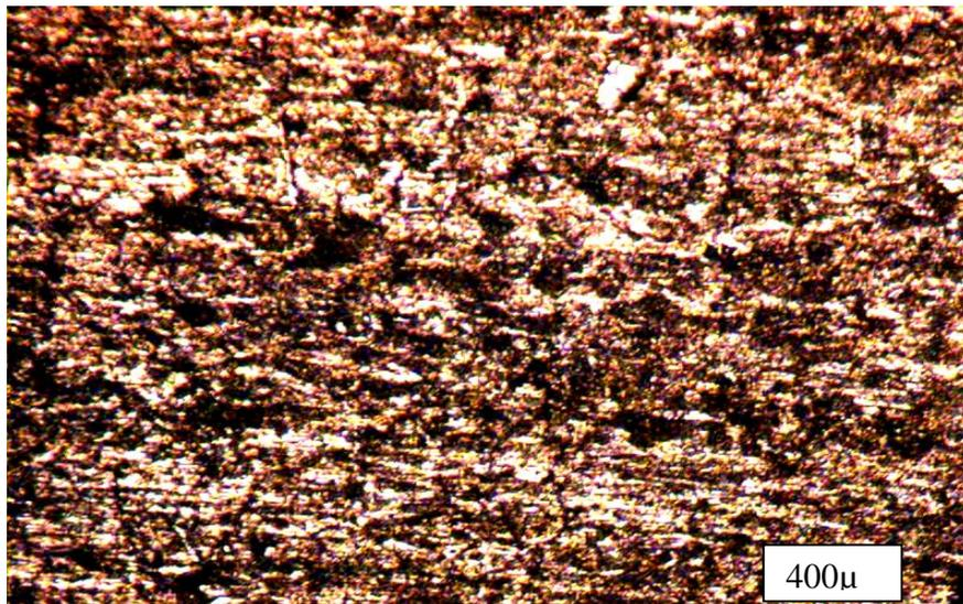
**Plate 4.3 Micrograph of etched Aluminum test sample using Tagwai Dam sand**
