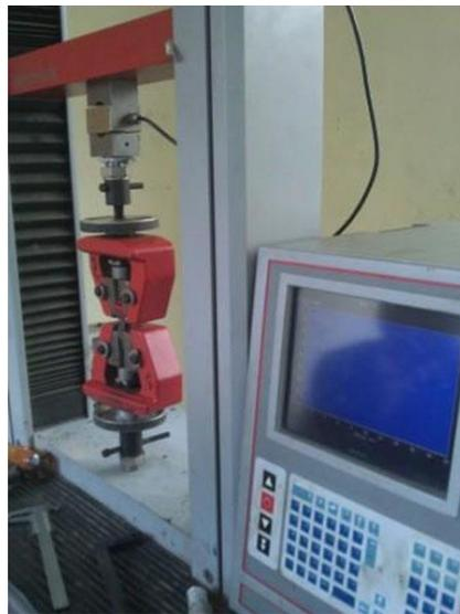
**Plate 2.4: Universal Testing Machine, FIRO Laboratory**
