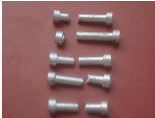
**Plate 3.5: Aluminium Cast Samples after Tensile Tests**
