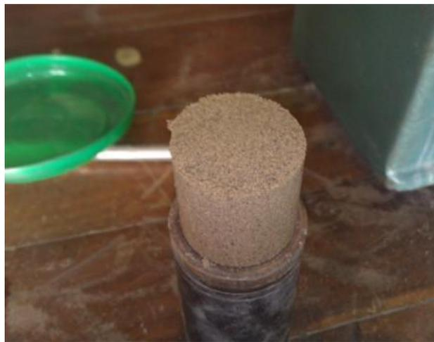
**Plate 3.1: 50 mm  $\times$  50 mm Sand Specimen**
