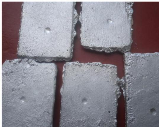
**Plate 3.6: Aluminium Cast Samples Showing Indentation of Hardness Tests**
