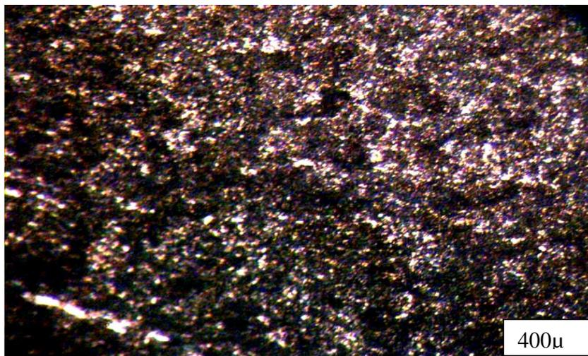
**Plate 4.2 Micrograph of etched Aluminium test sample using Tungan Mallam sand**
