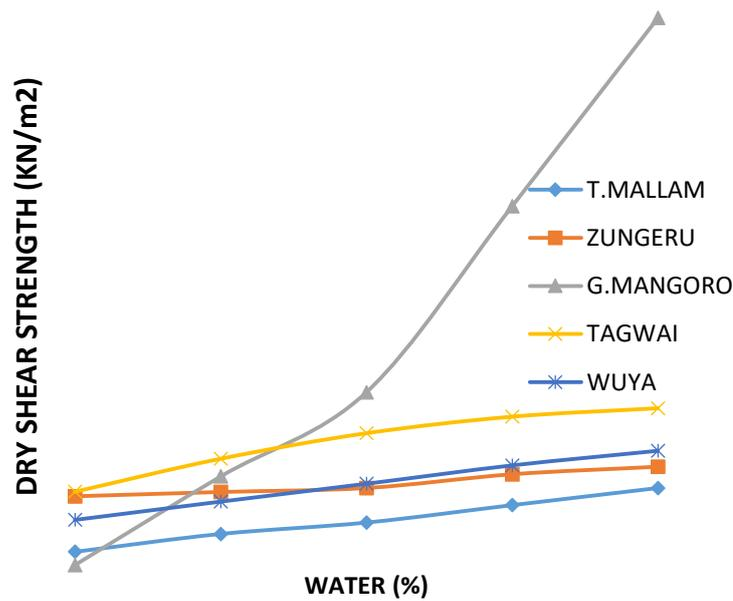
**Figure 4.6: Variation of Dry Shear Strength with Water Content**
