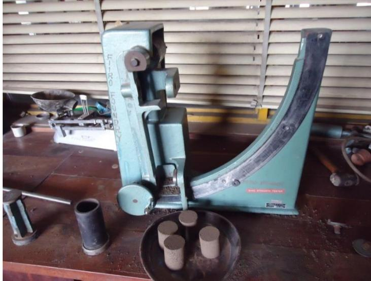
**Plate 2.1: Ridsdale-Dietert Universal Sand Strength Machine, FIRO Laboratory**
