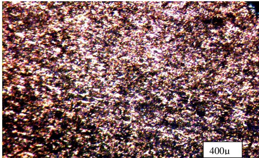
**Plate 4.4 Micrograph of etched Aluminium test sample using Wuya sand**
