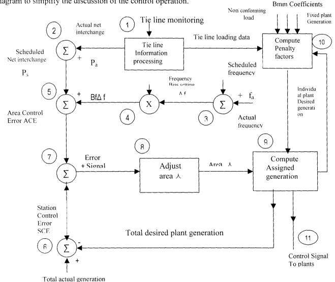
The larger circles on the diagram enclosing the symbols X or  $\Sigma$  indicates point of multiplication or algebraic summation of in coming signals.
