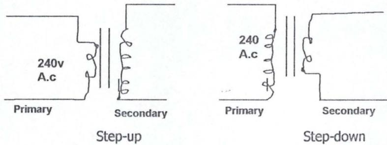
For this power supply the transformer used is a step down transformer since most modern electronic circuit operate at voltages well below 240v.
