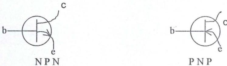
The bipolar transistor is made from silicon and germanium crystals. It has three regions that form the three distinct terminals such as Emitter (E) Collector (C) & Base (B).
