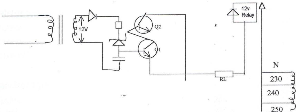
A voltage of 6.5v is maintained at the zener diode, which is the input voltage of the transistor. The output voltage is calculated using direct-coupled amplifier method. For directly coupled amplifier, the output is twice the input voltage i.e.  $V_o = 2V_i$ . So, since  $V_i = 6.5v$  therefore  $V_o = 2 \times 6.5 = 13v$ . **This stabilizer is designed to deliver 500w**, so the current (I) will be power divided by voltage, which is equal to 2.08A (i.e.  $P/V = 500/240$ )
