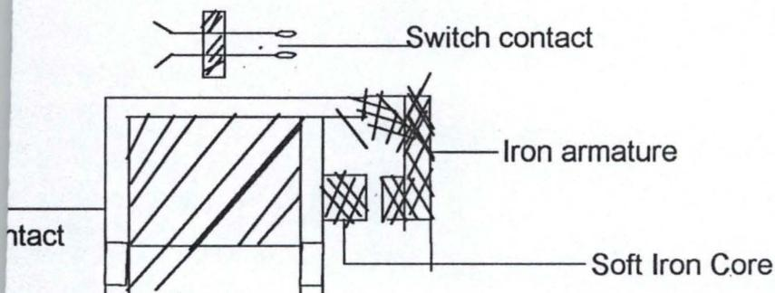
Fig. 1.8 (a): The diagram of a relay
