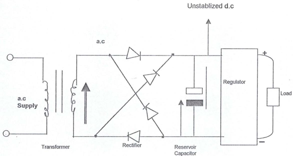
Block arrangement of a typical mains-operated d.c power supply.
