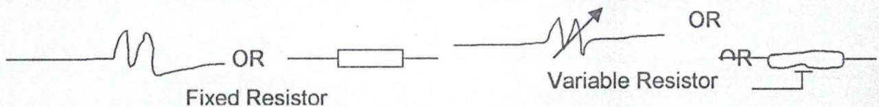
**Ratings:** – Resistors are rated in Ohms and the wattage determined by the size. The manufacturer often gives this. The Ohmic values of resistors are calculated using Colour codes. Below is an illustrative example:
