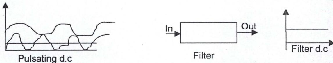
A circuit that converts a pulsating output from a rectifier into a very steady dc level is known as **filter** because it filters out or smoothens out the pulsation in the output. There are many types of filter circuits such as the LR filter, LC filter, C-L-C filter (PC), shunt capacitor filter e.t.c. But shall be concentrating on the shunt capacitor filter.
