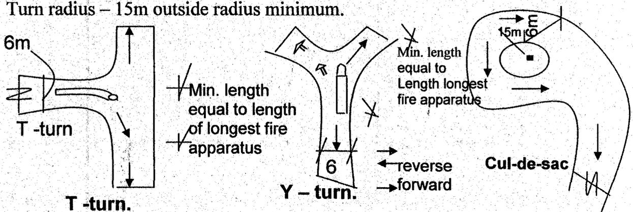
**Figure 3:6** Turning Radius access for fire apparatus.
