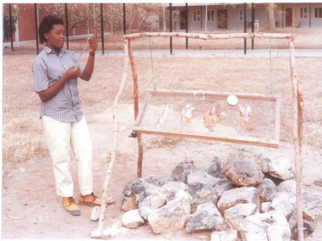
Plate II: Solar dryer rocks, rack and measurement of some parameters.
