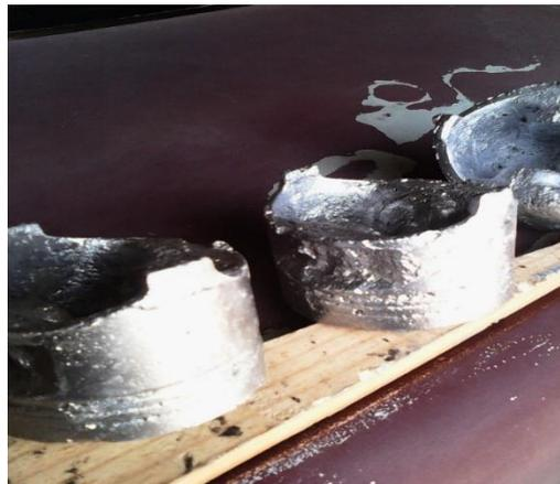
**Plate V: Cast Composite Piston**
