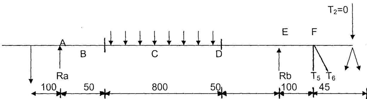
Fig. 10: Loading on Cylinder Shaft
