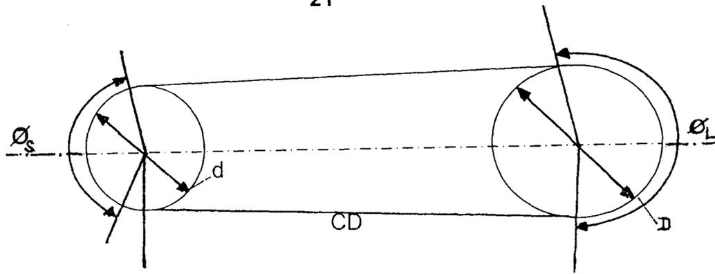
Fig. 5: Showing angles of rap for winnow and blower pulleys
