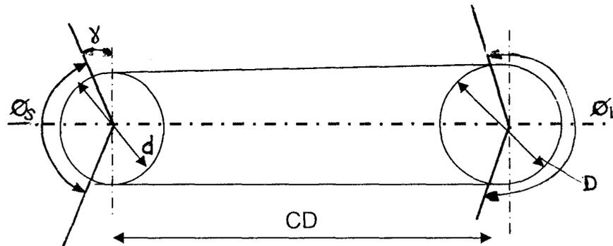
Fig. 4: Showing angles of rap for blower and cylinder pulleys.
