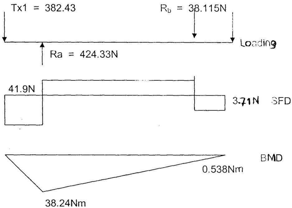
Fig. 14: Cylinder Shaft Loading Condition, Shear Force Diagram
