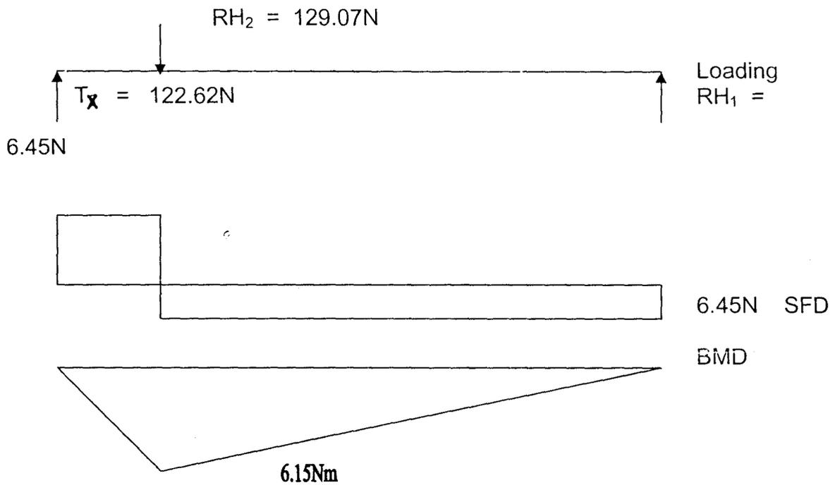
Fig. 9: Shaft Loading condition, shear free diagram and bending moment diagram in horizontal condition
