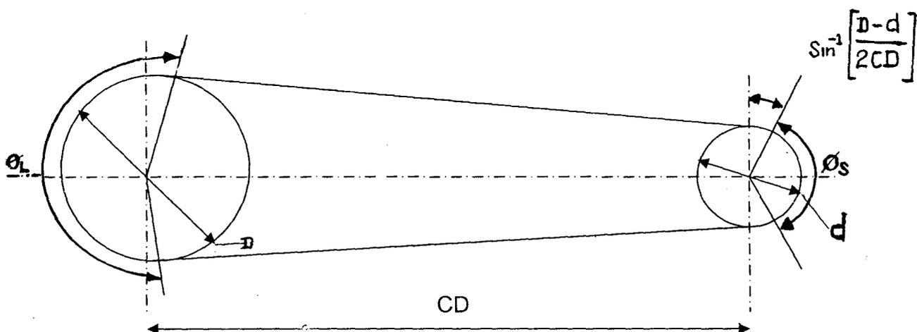
Fig. 3: Showing angles of rap for motor - cylinder pulleys
