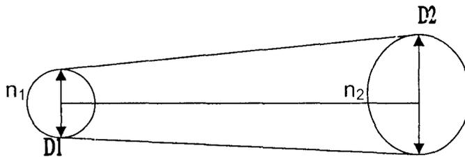
Fig. 2: The Peripheral Velocities on pulleys
