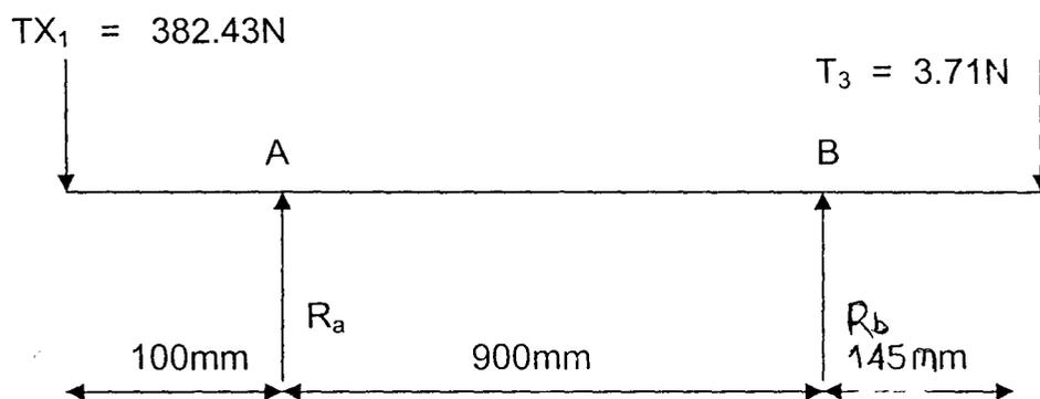
Fig. 13: Loading of Cylinder Shaft in Horizontal direction
