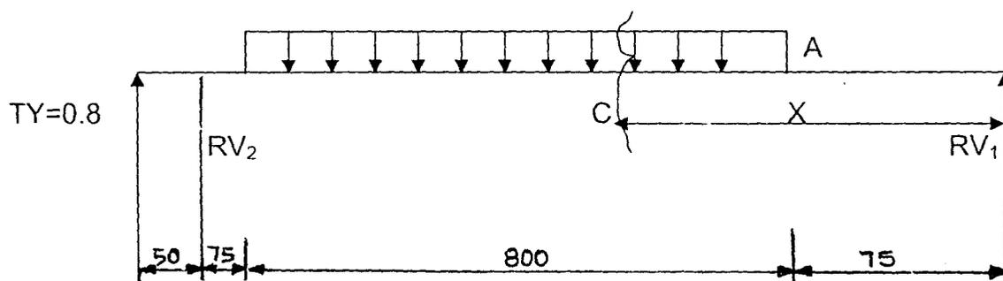
Fig: 6: Shaft Load Distribution in the Vertical Direction
