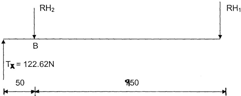
Fig. 8: Shaft Load Distribution in the Horizontal Direction
