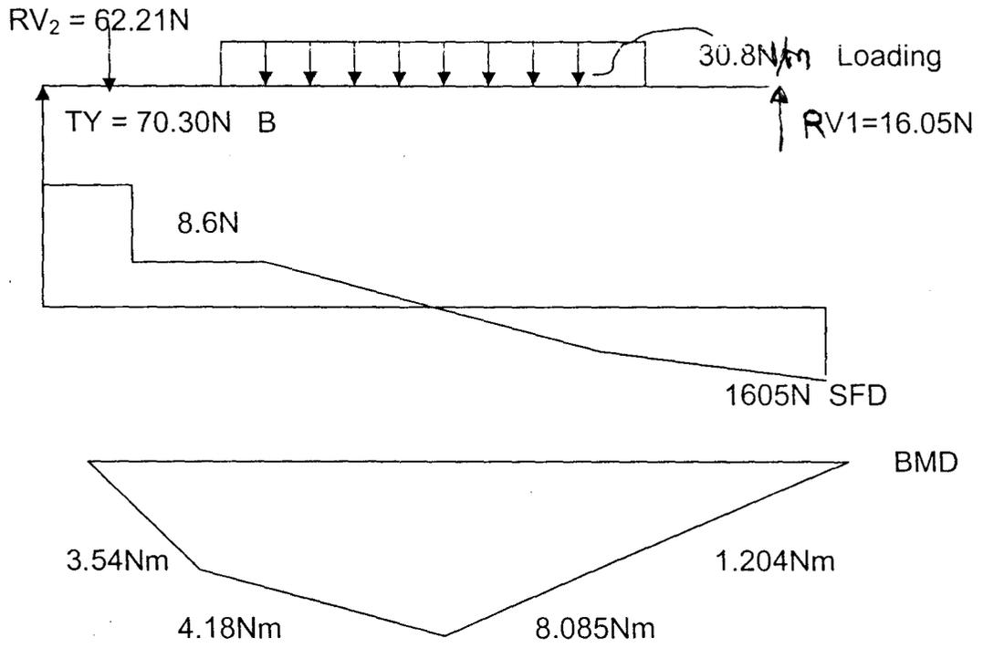
Fig. 7: Showing shaft loading, shear force diagram and bending moment diagram in vertical direction
