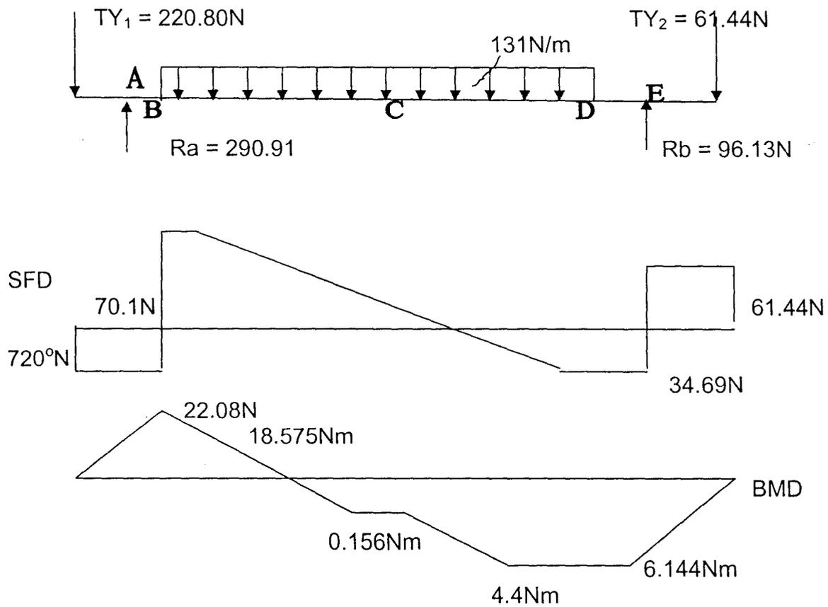
Fig. 12: Showing the loading, shear force and bending moment diagram in vertical direction for cylinder shaft.
