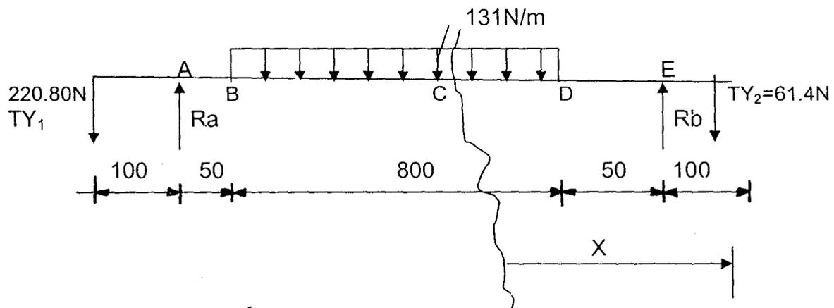
Fig. 11: Vertical Load distribution
