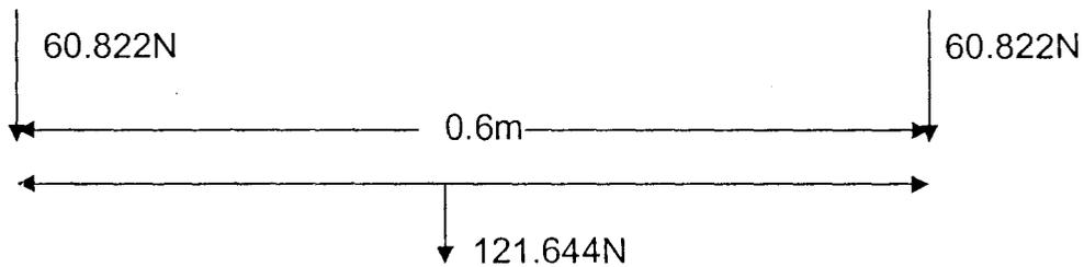
Fig. 16: Loading on the frame
