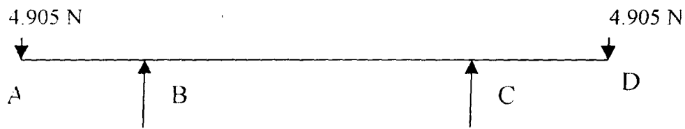
Fig. 3.8 free body diagram of gear output shaft.
