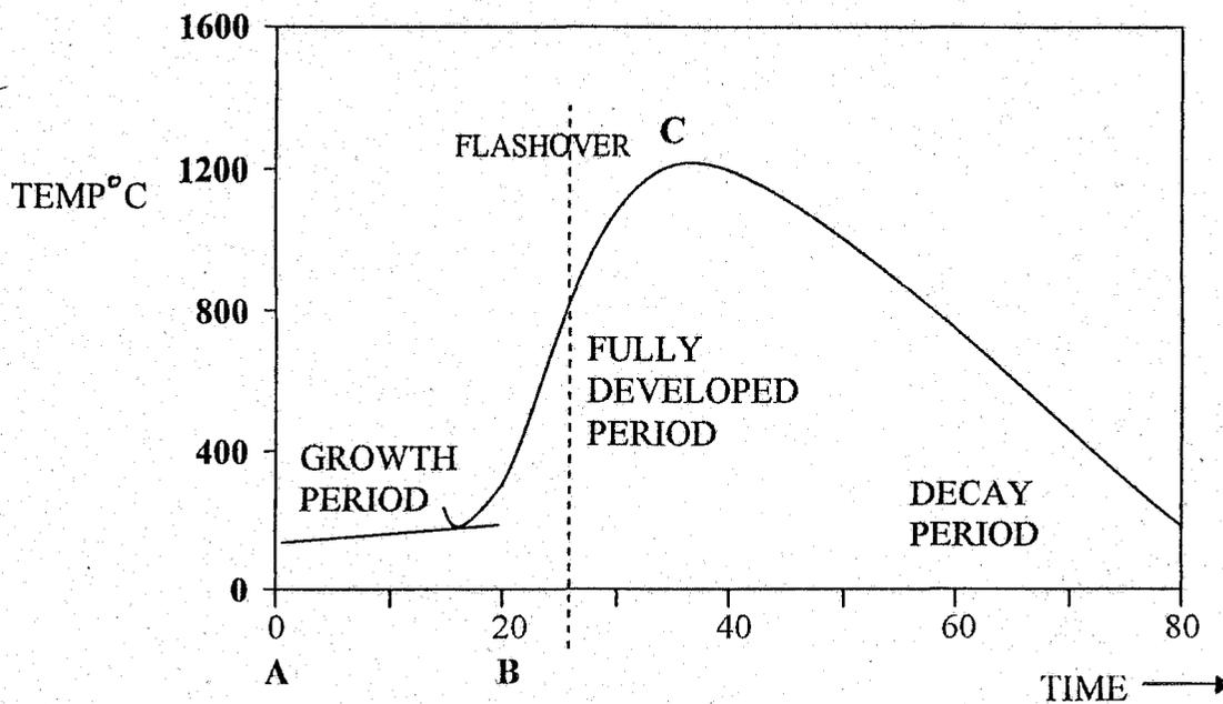
FIG.3.1: Time/temperature fire profile.
