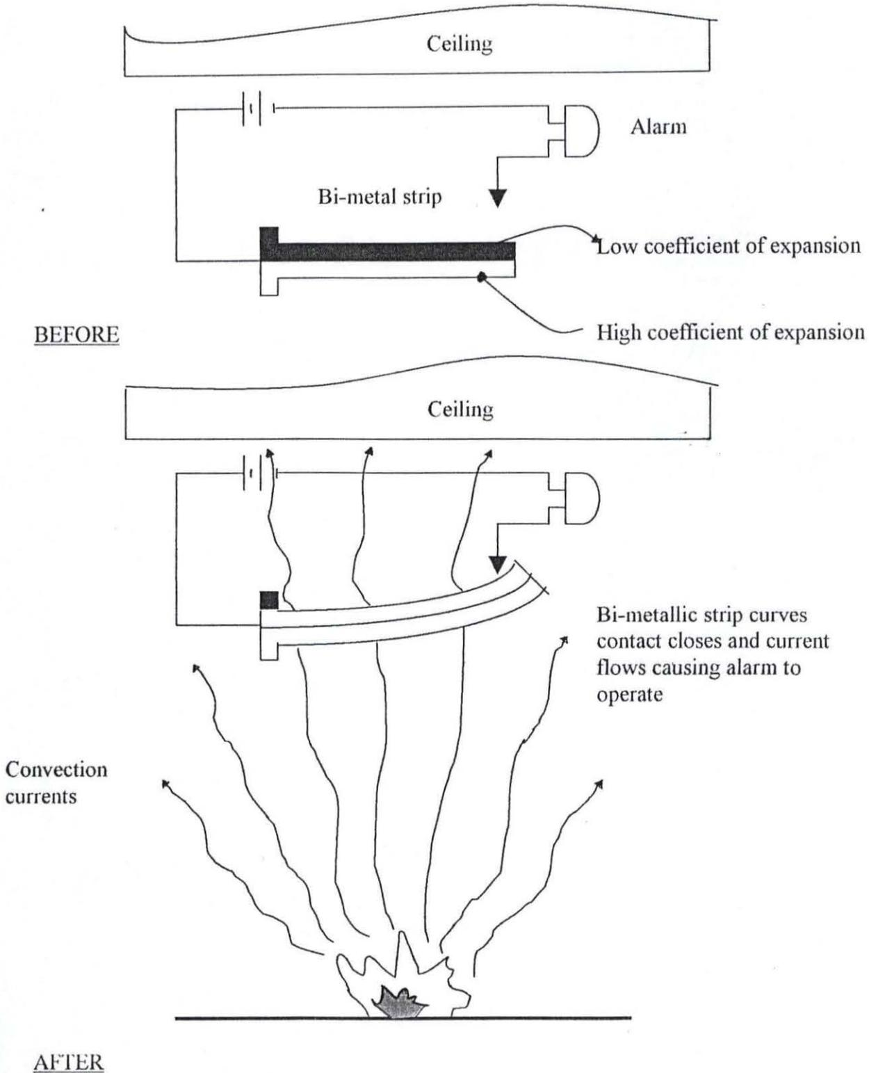
FIG. 3.2: Bimetallic strip heat detector
