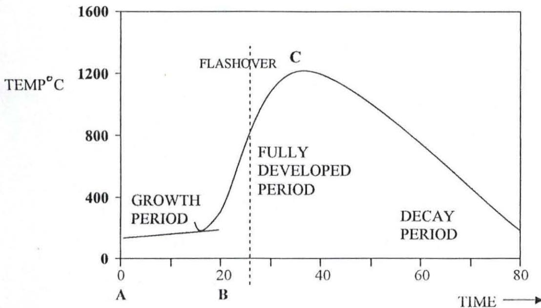
FIG.3.1: Time/temperature fire profile.
