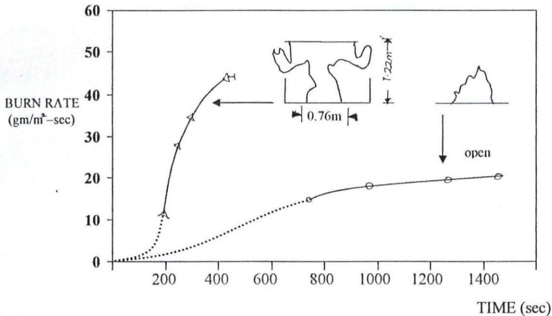
FIG. 3.0: Effect of enclosure on the burning rate of a square polymethyl methacrylate slab.
