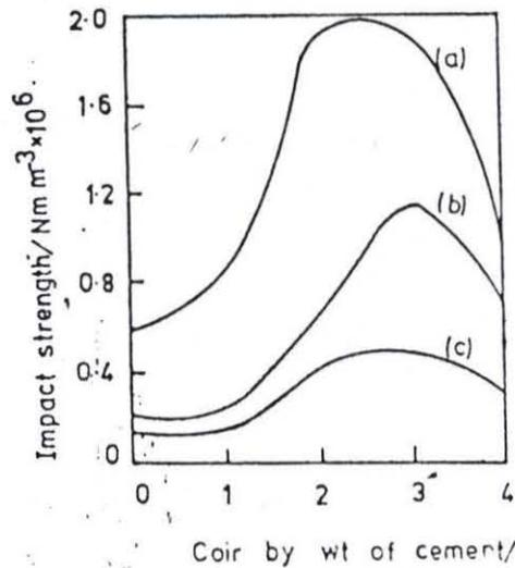
Variation with coir content of impact strength of coir-reinforced concrete beams at different ages. Beams aged for 90 days (a), 21 days (b) and 7 days (c).
