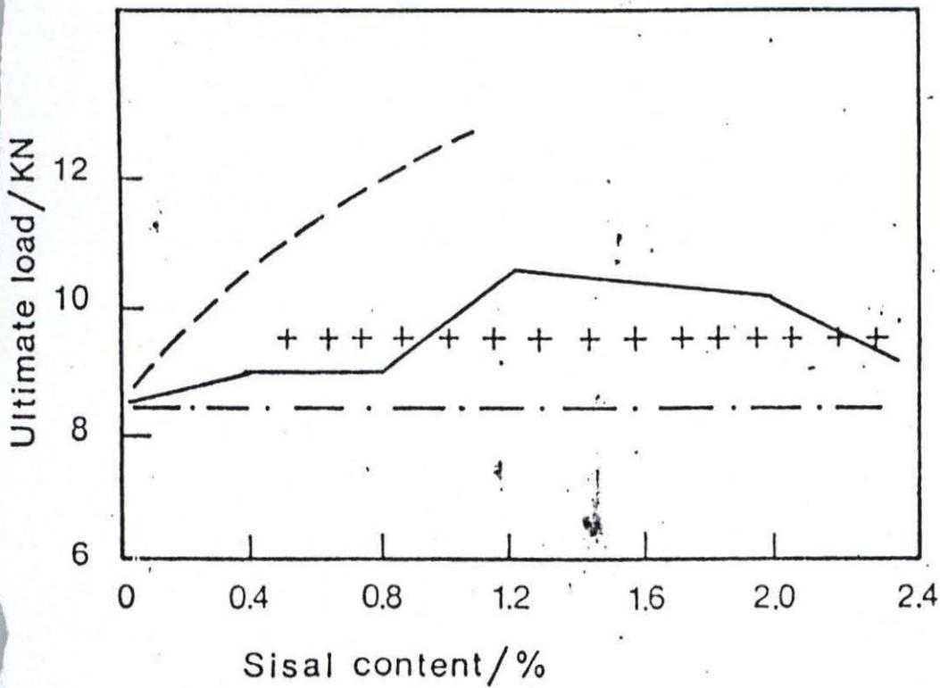
Sisal-reinforced concrete beam flexural strength tests after aging for 28 days (4)
