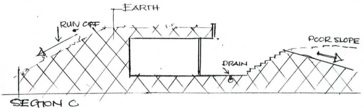
while Section B shows a cut-off gravel trench with drain tile at the base. Section C illustrates some drainage problems associated with sunken courtyards which are common in earth sheltered designs. It is preferable for the surrounding ground to slope away from the structure on all sides, then only the rainfall which falls directly into the court must be handled by a drainage system.
