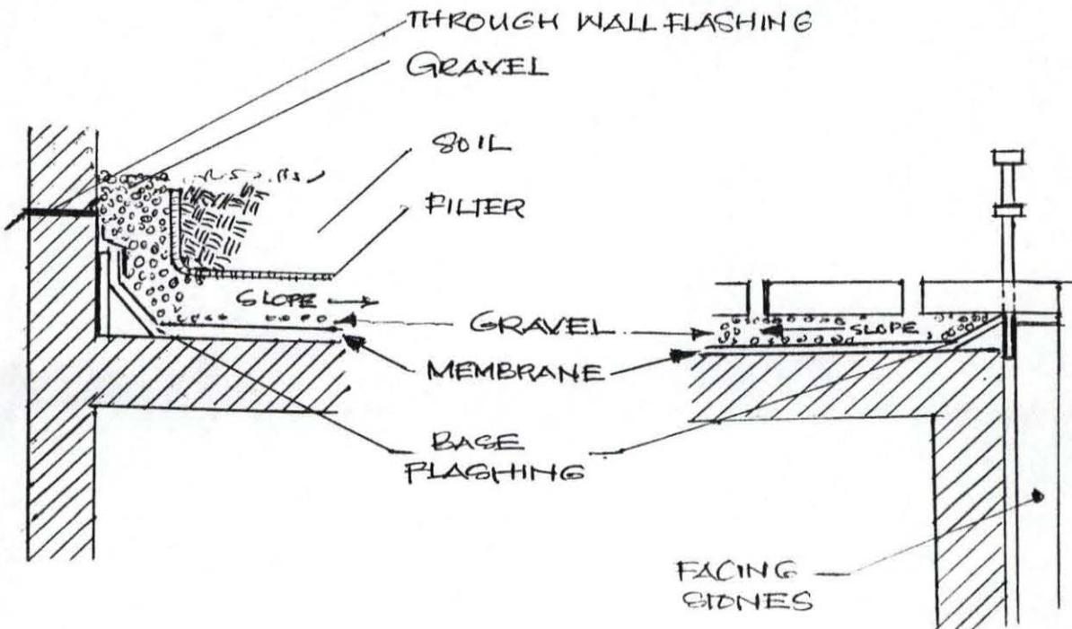
More so, the details are important to the success of a roof terrace, and in some instances the walls of the building as well. Typical schematic details are shown in figure below where the membrane is arranged to carry water away from the walls.
