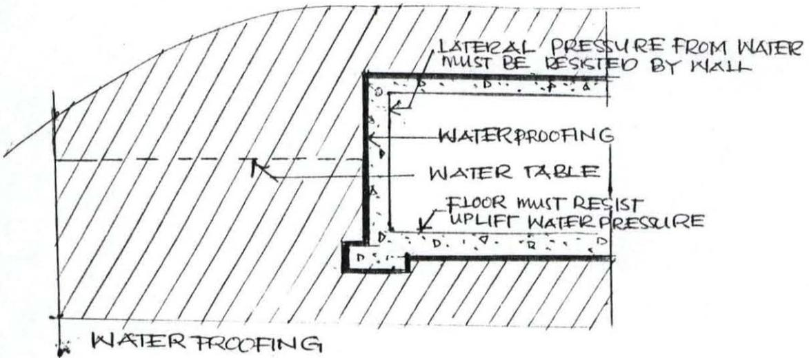
proofing technique would be needed to stop any capillary draw moisture into the wall. When temporary pressure cannot be eliminated, and this could rarely be guaranteed, damp-proofing will not surface for complete protection because damp-proofing is not designed to keep out water under pressure. Diagrams below show in the best language of architecture, what need to be done.
