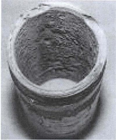
Plate x. Crevice Corrosion. ([www.corrosion-club.com](http://www.corrosion-club.com))
