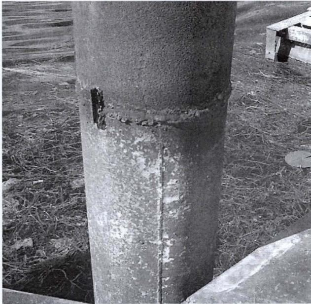
Plate xi. Uniform Corrosion on oil well pipe. ([www.corrosion-club.com](http://www.corrosion-club.com))
