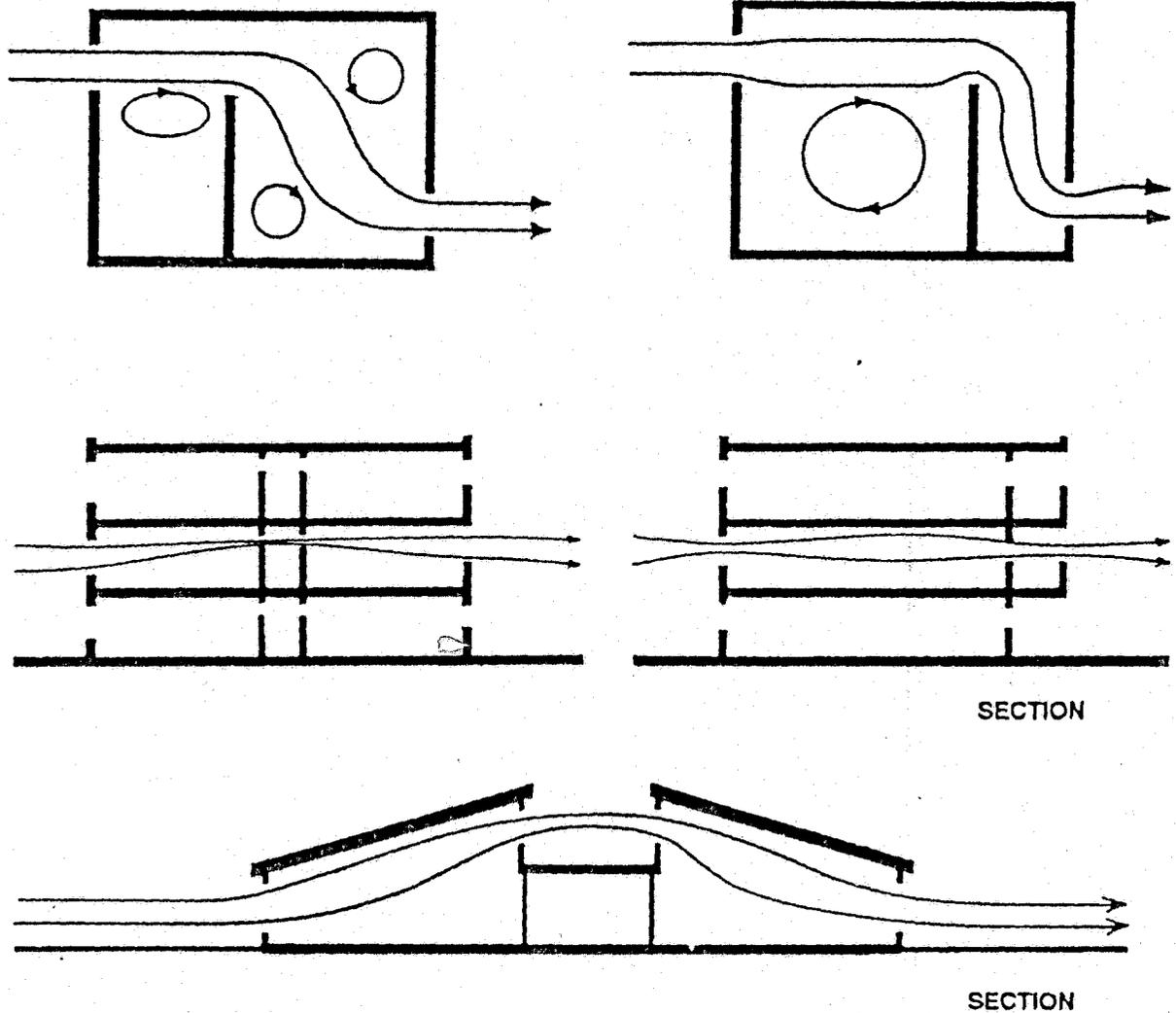
FIG 3.58 Explains THE DEPTH OF A ROOM WHICH HAVE EFFECT ON VENTILATION. OPEN PLANS MOST ESPECIALLY IN THE WARDS WHERE PATIENTS STAY, ARE PREFERABLE BECAUSE PARTITIONS INCREASE THE RESISTANCE TO AIR FLOW AND THEREBY DECREASE TOTAL VENTILATION
