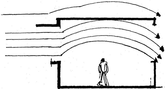
A SOLID HORIZONTAL OVERHANG PLACED HIGH ABOVE THE WINDOW STRAIGHTENS OUT THE AIR STREAM.
