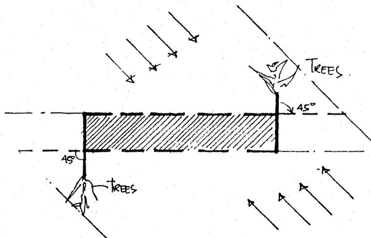
DEFLECTING WALLS AND VEGETATION CAN BE USED TO CHANGE AIR FLOW DIRECTION SO THAT THE OPTIMUM SOLAR ORIENTATION CAN BE MAINTAINED.
