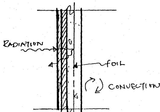
\* THIS FOIL WHEN PLACED IN THE CENTRE, OF AN AIR SPACE IT WILL ALSO SLIGHTLY REDUCE HEAT FLOW BY CONVECTION!
