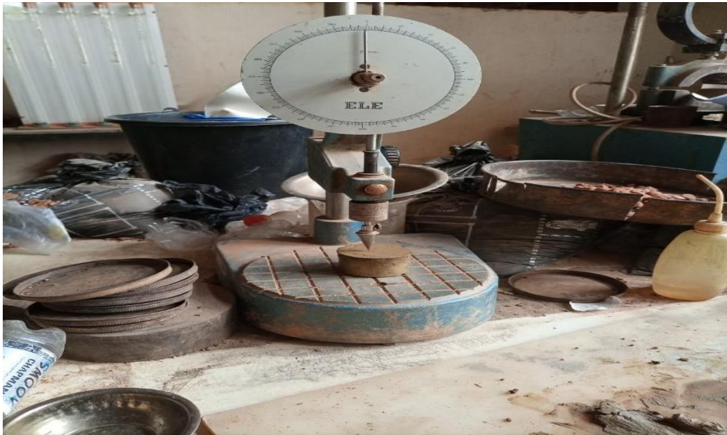
Plate VII: Cone Penetration Test Apparatus
