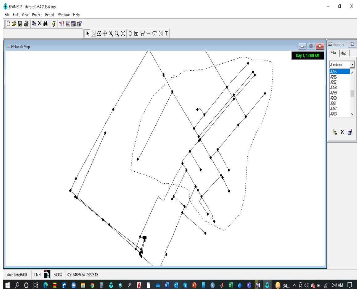
**Figure 3.10:** EPANET interface of Shiroro DMA showing the selected nodes for analysis (allow EPANET to distinguish nodes, rather plane dots)
