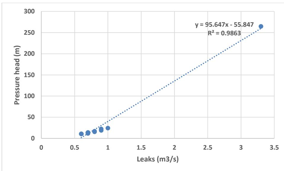
**Figure 4.4: Pressure and leak relationship**
