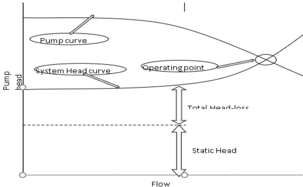
**Figure 2.2:** Relationship between pump and system curve
