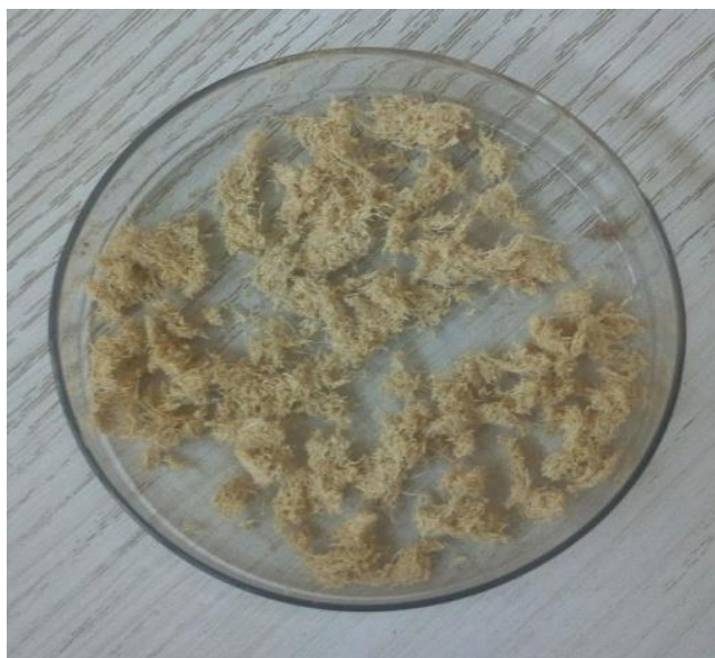
Plate V: Image of BPFs, after bleaching with sodium chlorite ( \text{NaClO}_2 )
