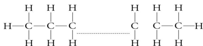
Figure 2.9: Molecular structure of polyethylene
