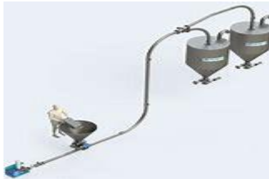
Plate 2.2: A Dilute Phase Pneumatic Conveying System
