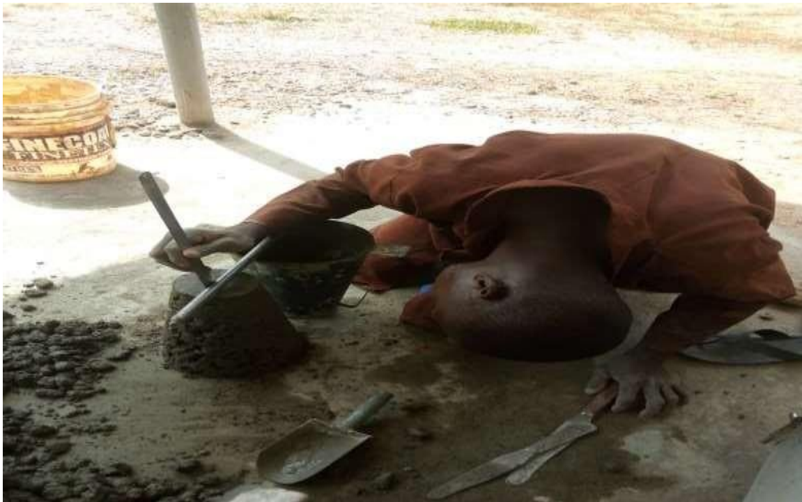
Plate XII: Slump testing in Federal Poly Bida Civil Engineering Laboratory
