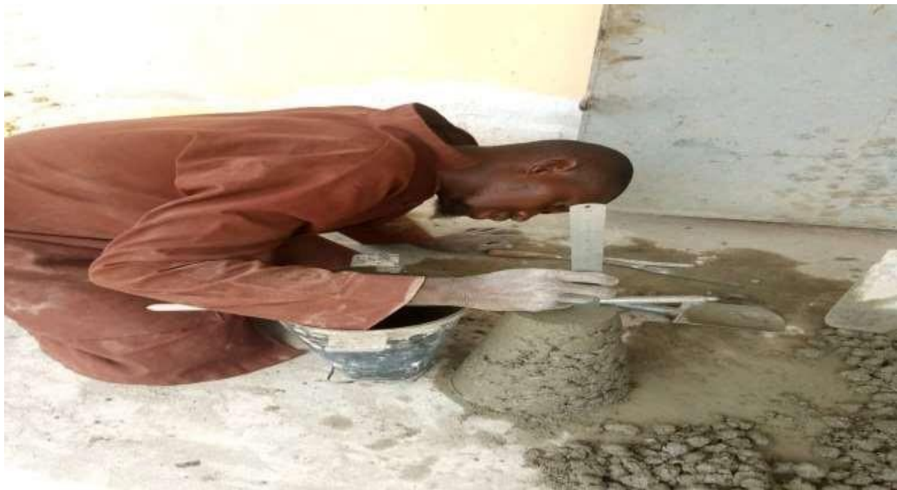
Plate XIII: Slump test in Federal Poly Bida Civi1 Engineering Laboratory
