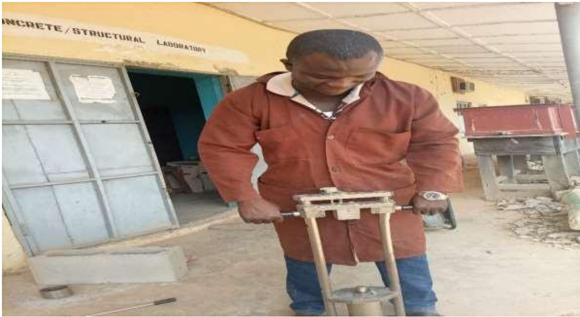
Plate VI: Aggregate crushing value test
