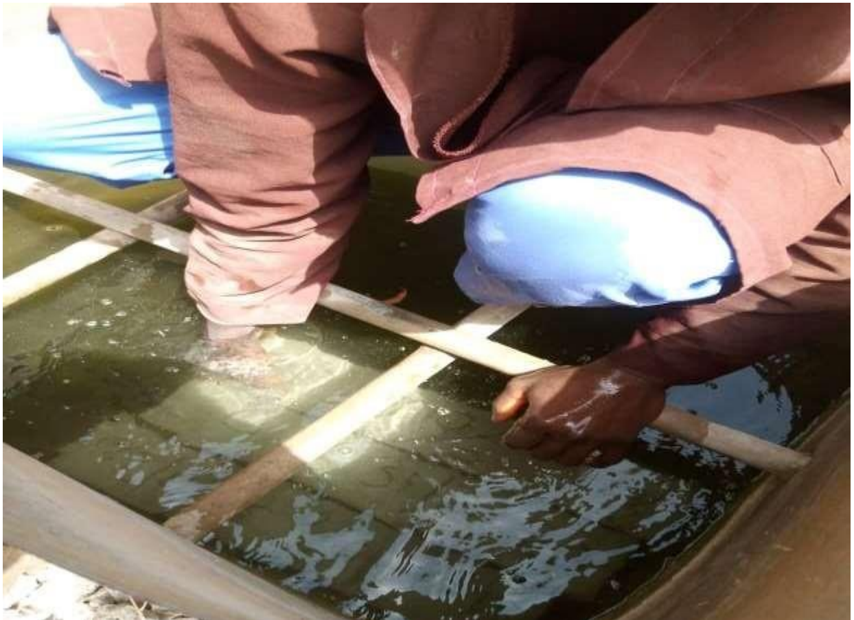
Plate XVIII: Curing of concrete sample at Federal Poly Bida Civil Engineering Laboratory
