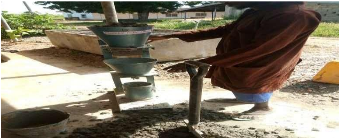
P1ate XVII: Compacting factor test at Federal Poly Bida Civi1 Engineering Laboratory
