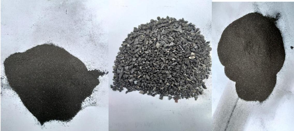
**Plate III:** Three sieve sizes of manganese samples
