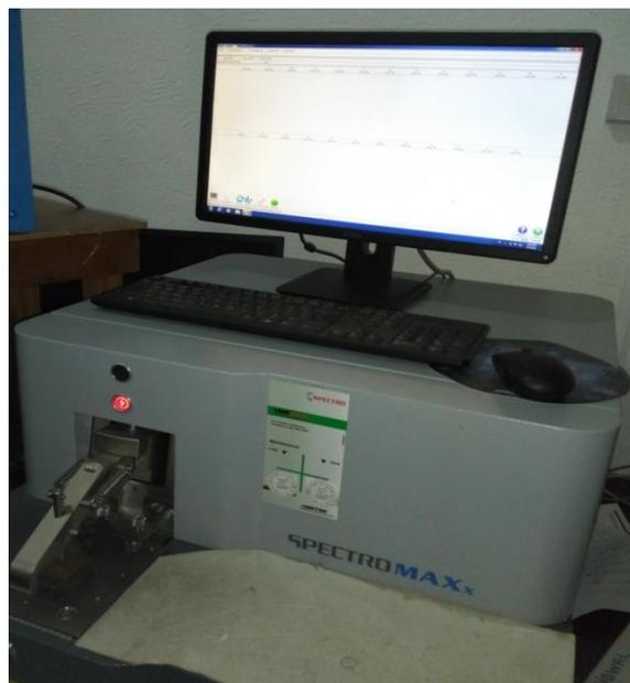
Plate X: Optical Emission Spectrometer (OES)
