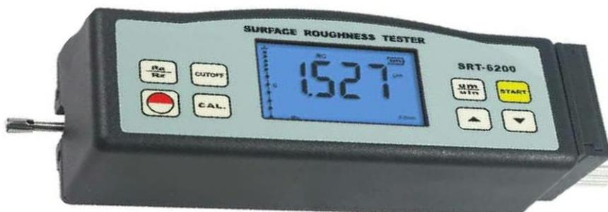
Plate IV: Digital surface roughness tester
