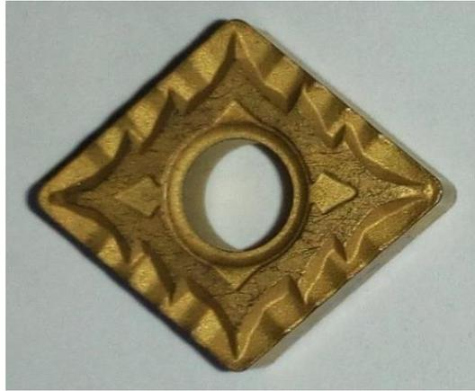
Plate II: Cutting tool insert
