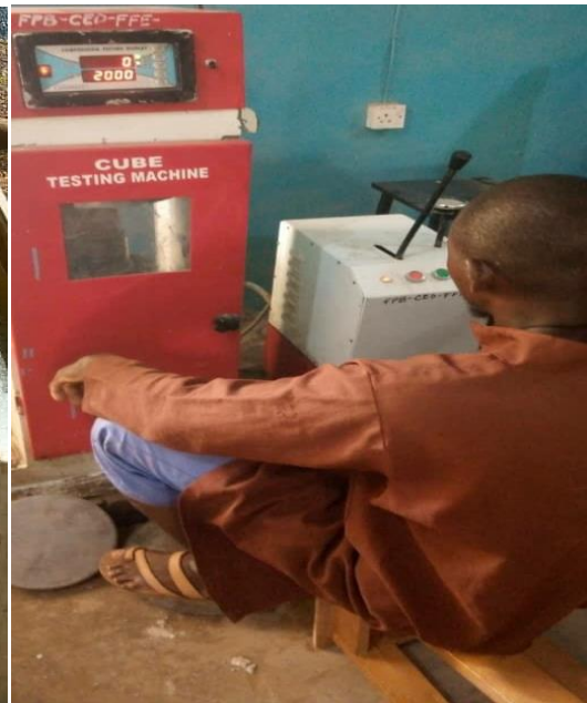
Plate V: Crushing of concrete cubes
