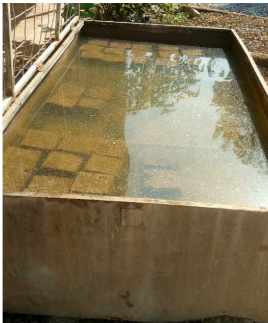
Plate IV: Curing of concrete cubes
