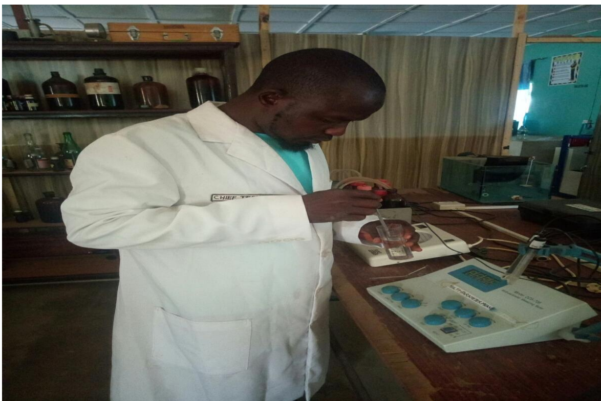
Plate VIII: Determination of Electrical Conductivity and Temperature using multiparameter apparatus
