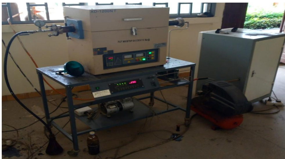
Plate VIII: Experimental Setup for Hydrous Pyrolysis and Anhydrous Pyrolysis (FUT Minna, Step B)
