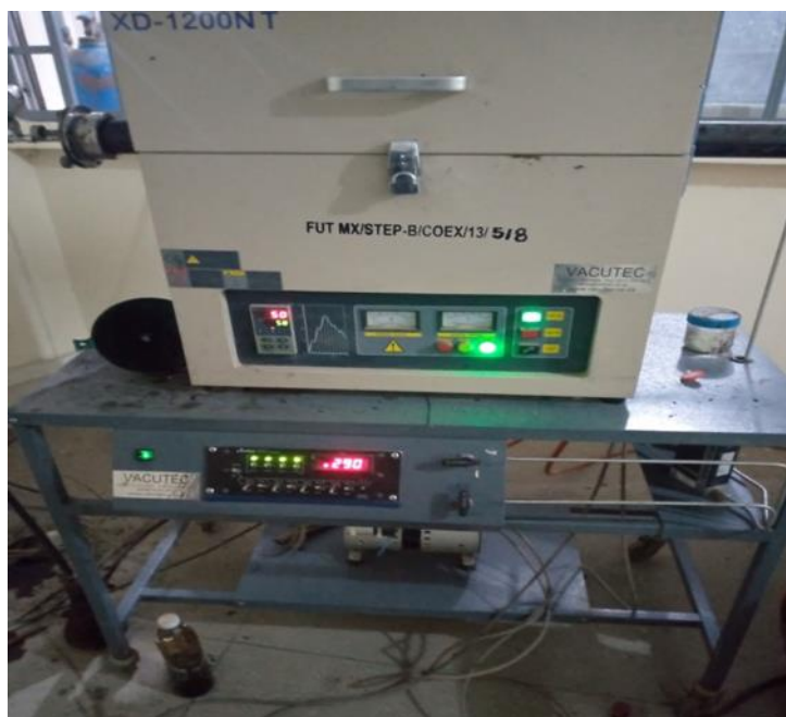
Plate IX: Experimental setup during a run showing the inert gas flow rate of 290 mL/min (FUT Minna, Step B)
