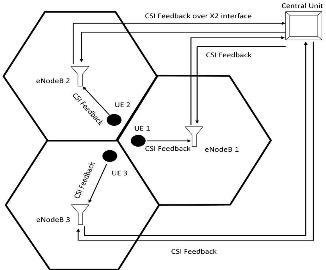
**Figure 2.1: The Centralised Joint Transmission Architecture (adapted from Kazi and Wainer, 2020)**
