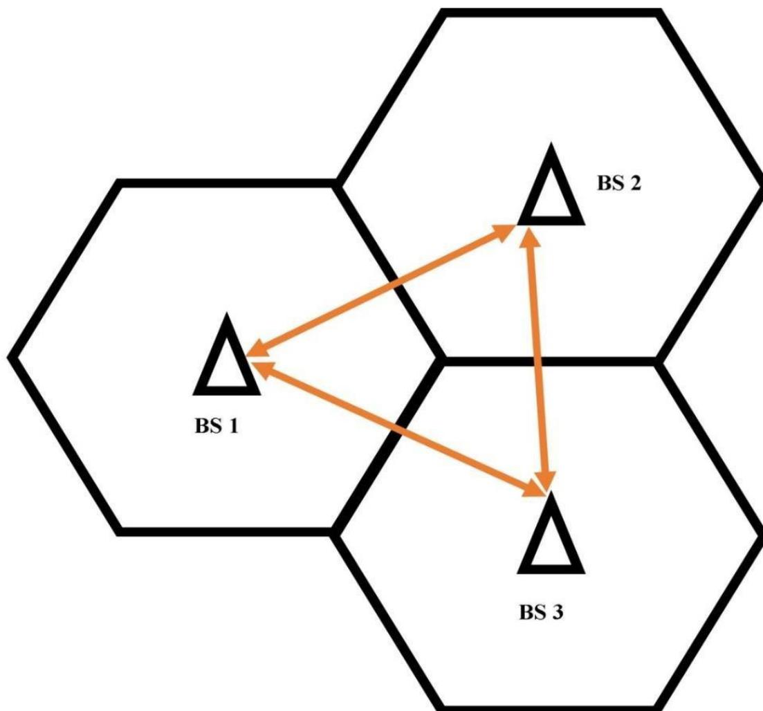
**Figure 2.3: Cluster of Base Stations (adapted from Li *et al.*, 2013)**
