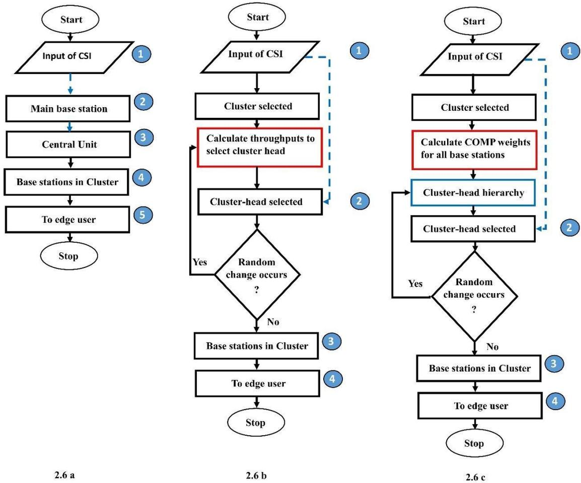
**Figure 2.6 a – c: Overview of the Coordinating Schemes (2.6a – The Centralised Architecture, 2.6b – The DCEC Architecture, 2.6c – The Developed Hierarchical Cluster-Head Table Architecture)**
