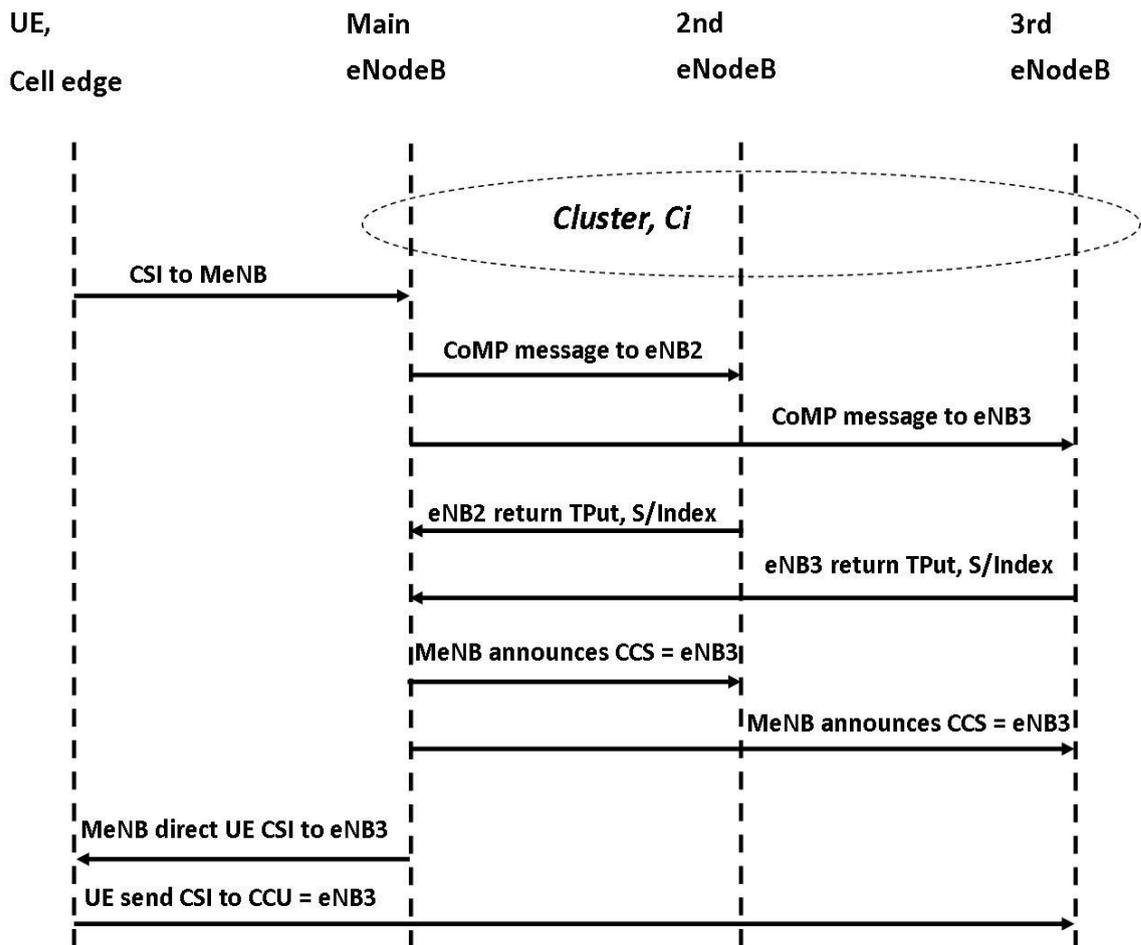
**Figure 3.4: Flow of COMP JT Command for the Hierarchical Scheme**
