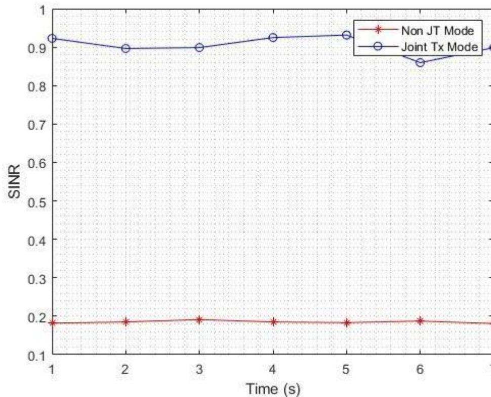
**Figure 4.7: SINR Comparison with Non-Joint Transmission Scheme**
