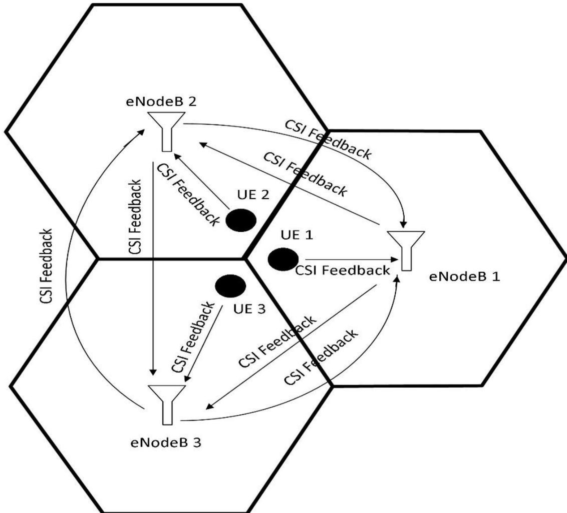
**Figure 2.2: The Distributed Joint Transmission Architecture (Adapted from Kazi and Wainer, 2020)**
