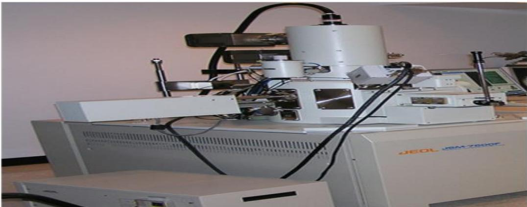
**Plate VII:** Picture of Scanning Electron Microscopy Machine
