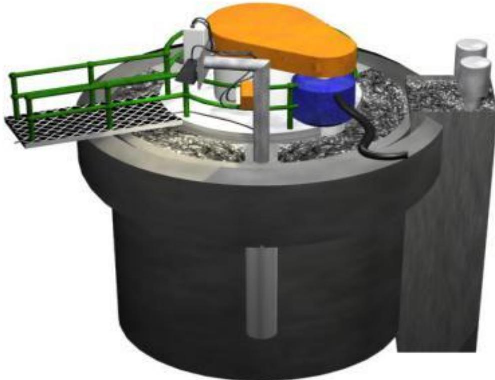
**Figure 2.1:** Illustrates cylindrical froth flotation cell (Cheraghian *et al.*, 2018)
