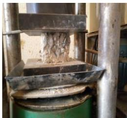
**Plate 9:** Plain concrete cube under compression machine
