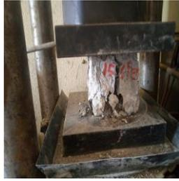
**Plate 11:** Failure mode of concrete cube under compression machine
