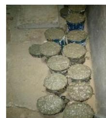
**Plate 20:** fresh concrete in cylinder mould
