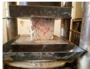
**Plate 10:** 5% PET concrete cube under compression machine
