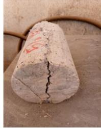
**Plate 13:** Failure mode of 5% PET concrete cylinder specimen
