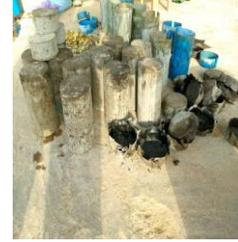
**Plate 22:** Demoulding of concrete samples from mould
