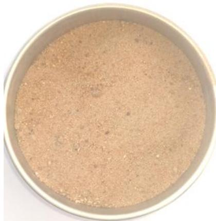
**Plate III:** River sand as fine aggregate
