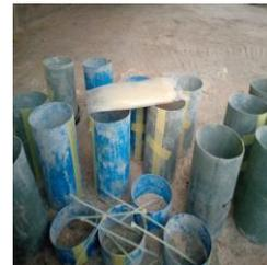
**Plate 6:** PVC cylinder mould
