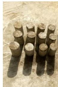
**Plate 15:** Plain and PET concrete cylinder specimen
