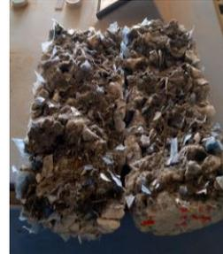
**Plate 14:** Failure mode of PET concrete cylinder specimen
