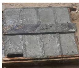
**Plate 19:** fresh concrete in cube formwork
