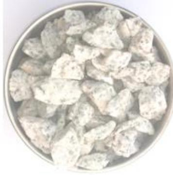
**Plate II:** Crushed granite stone as coarse aggregate
