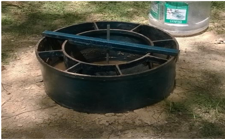
Plate I: The Double Ring Infiltrometer having 300 mm inner diameter and 600 mm outer diameter (ASTM, 2009).
