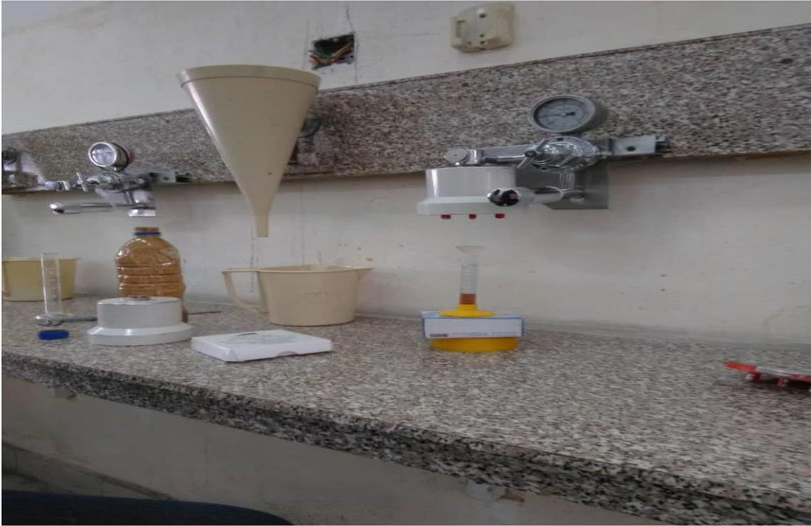
Plate A-7 Fluid loss setup
