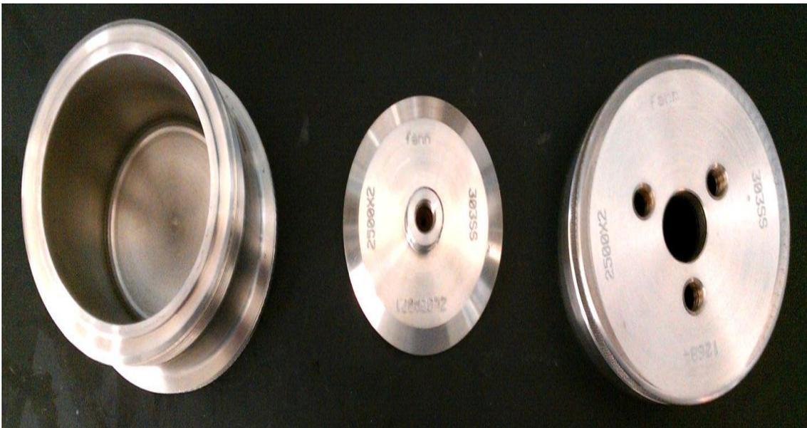
Plate A-4 Aging cell assembly
