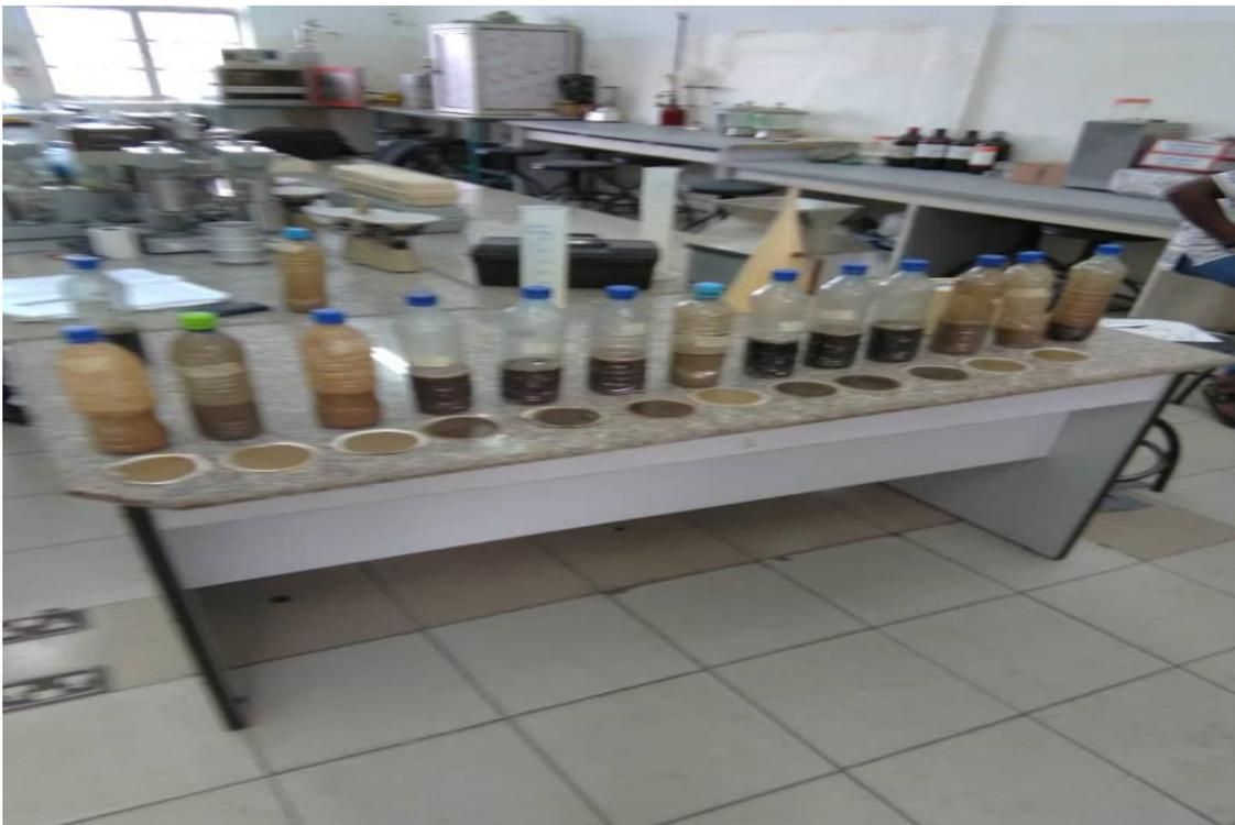
Plate A-8 Prepared drilling mud and their cake thickness
