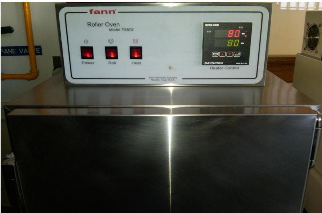
Plate A-6 Roller Oven in operation
