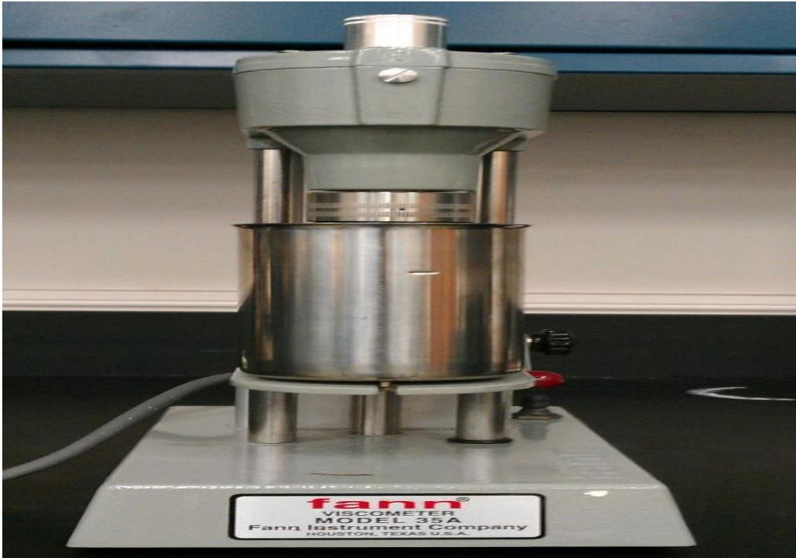
Plate A-1: Fann 35A Viscometer
