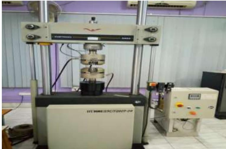
**Plate VI: Instron 8862 tensile machine**
