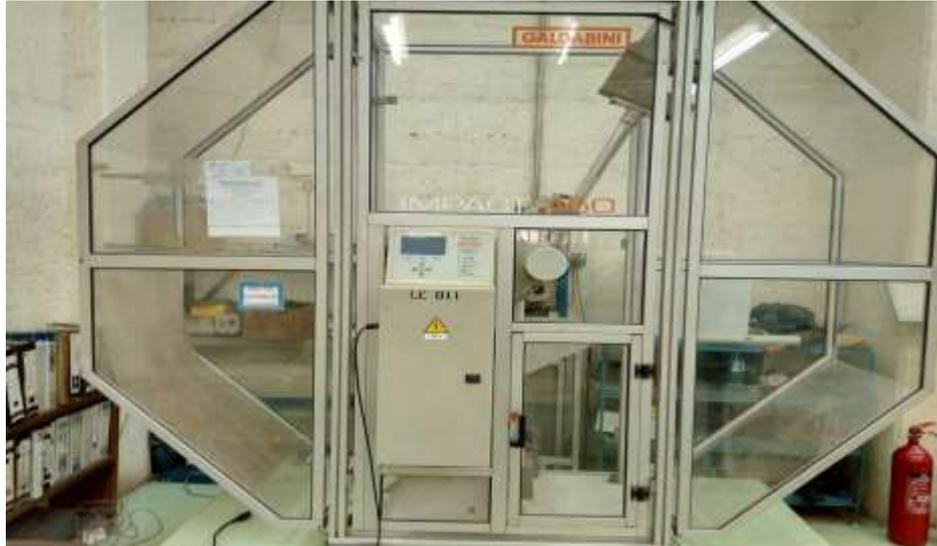
**Plate VII: Impact testing machine**
