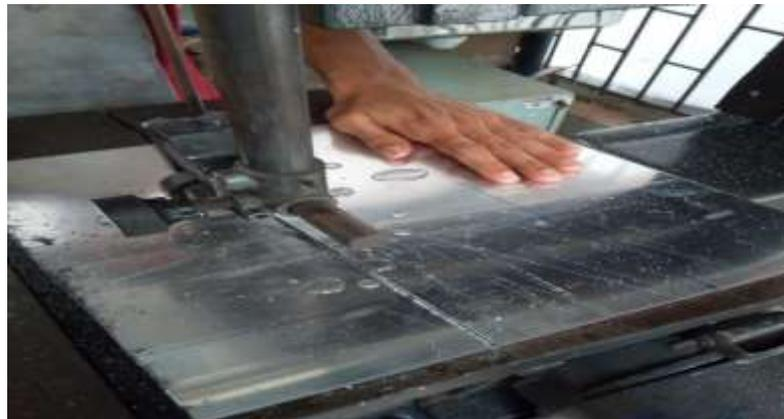
**Plate XI: Cutting of workpiece using band saw**
