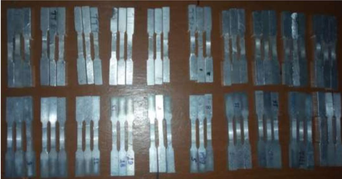
**Plate XIV: Tensile test specimens**
