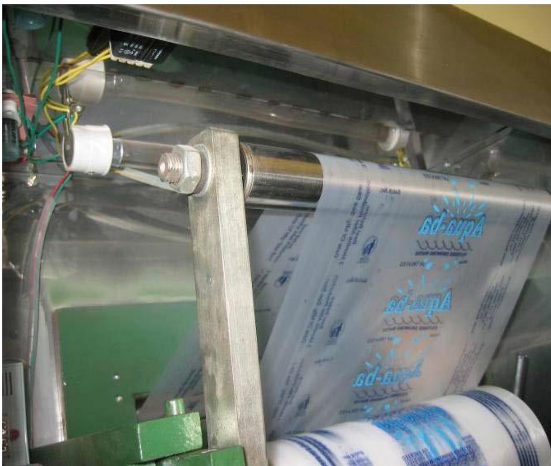
Plate II: UV-bulb in Sachet Machine used to Disinfect Polythene roll
