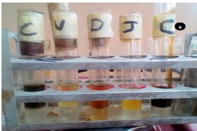
Plate I: Experimental set up for determination of emulsification of oils
