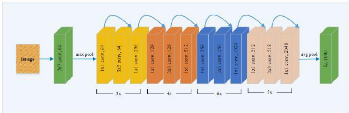
Figure 2.3: A Block Diagram Representation of Pre-trained Resnet-50 Architecture. (He et al. , 2016)
