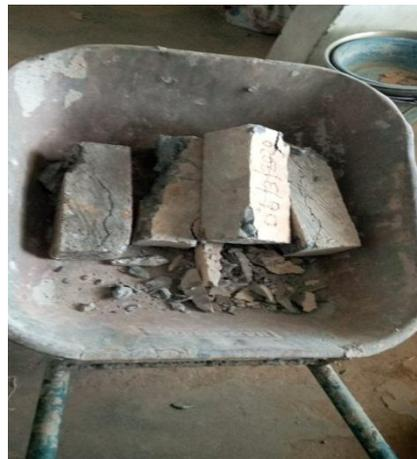
**Plate VI:** Crushed Concrete Columns
