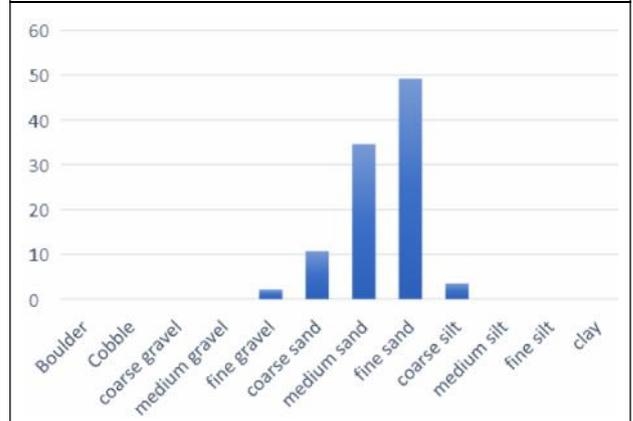
Figure 13: Bar Chart Representation of Grain Sizes in Samples Slump Site 4
