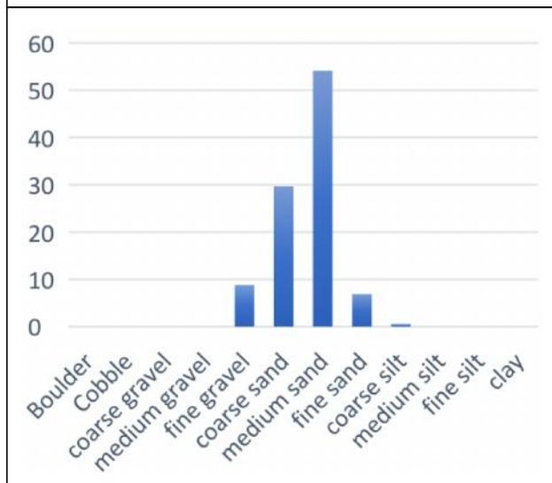
fine sand, coarse silt and fine gravel. Estimated values of  $C_u$  and  $C_c$  are 0.57 and 0.148 respectively, which indicates it is poorly graded. Table 5 is the sieve analysis result for slump site 3.
