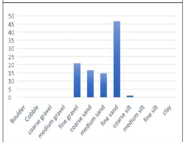
the sample contains high amounts of fine sand, medium to coarse sand and fine gravel. Estimated values of  $C_u$  and  $C_c$  are 5.31 and 0.711 respectively. The  $C_u$  reflects substantial amount of gravel, and is fairly graded.
