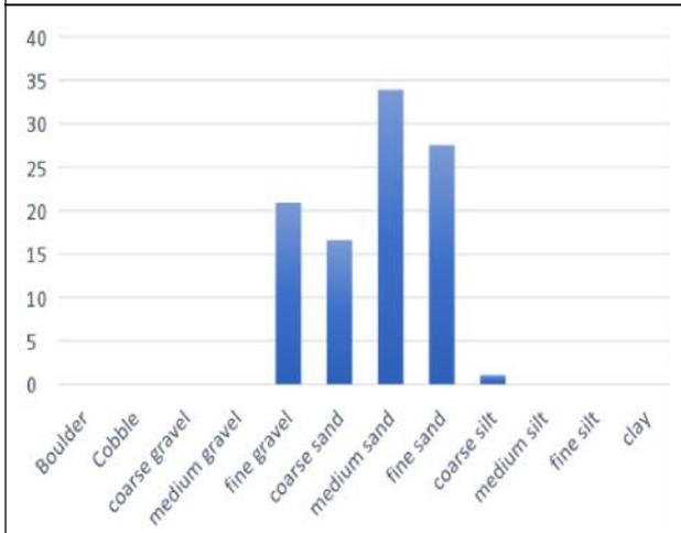
Figure 16: Plot of Percentage Mass Passing (PMP) versus Sieve Grain Size (Slump Site 6)
