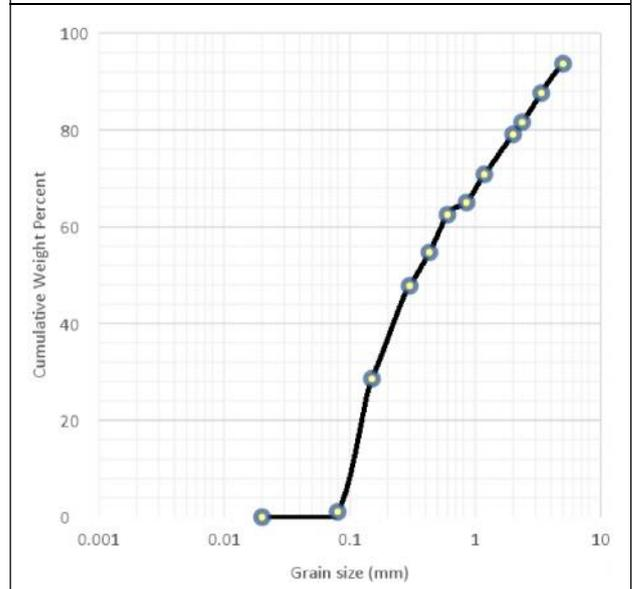
Figure 11: Bar Chart Representation of Grain Sizes in Samples Slump Site 3
