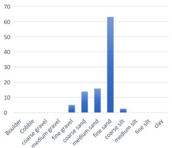
This indicates that the geological formation is poorly graded at this slump site. Table 4 is the sieve analysis result for slump site 2.
