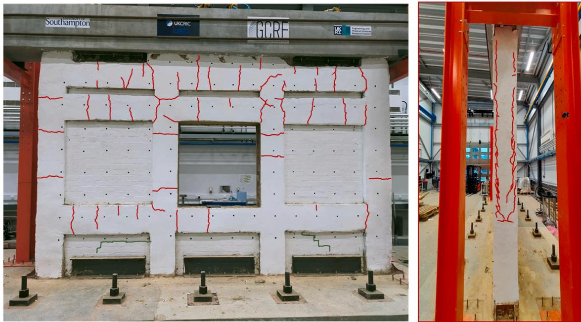
Fig. 9. Observed crack damage to the retrofitted wall at the end of the test.
