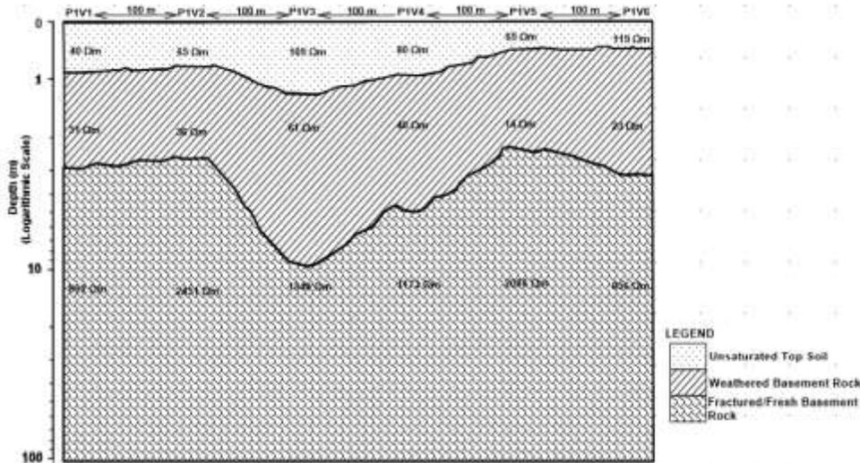
**Figure 8: Geoelectric/Geologic Section of Profile one**
