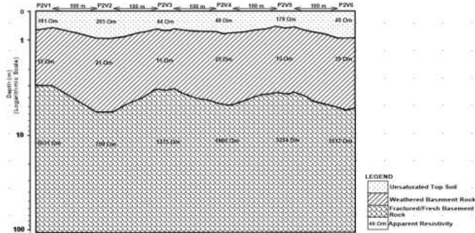
**Figure 9: Geoelectric/Geologic Section of Profile Two**
