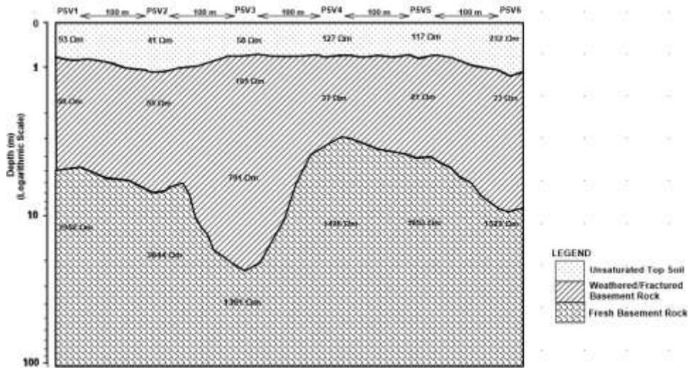
**Figure 12: Goelectric/Geologic Section of Profile Five**
