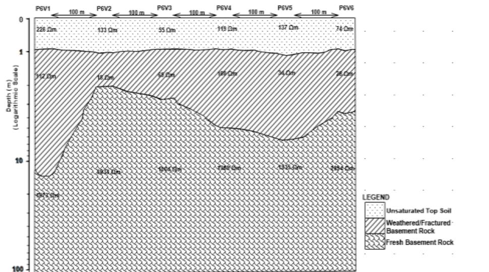
**Figure 13: Goelectric/Geologic Section of Profile Six**
