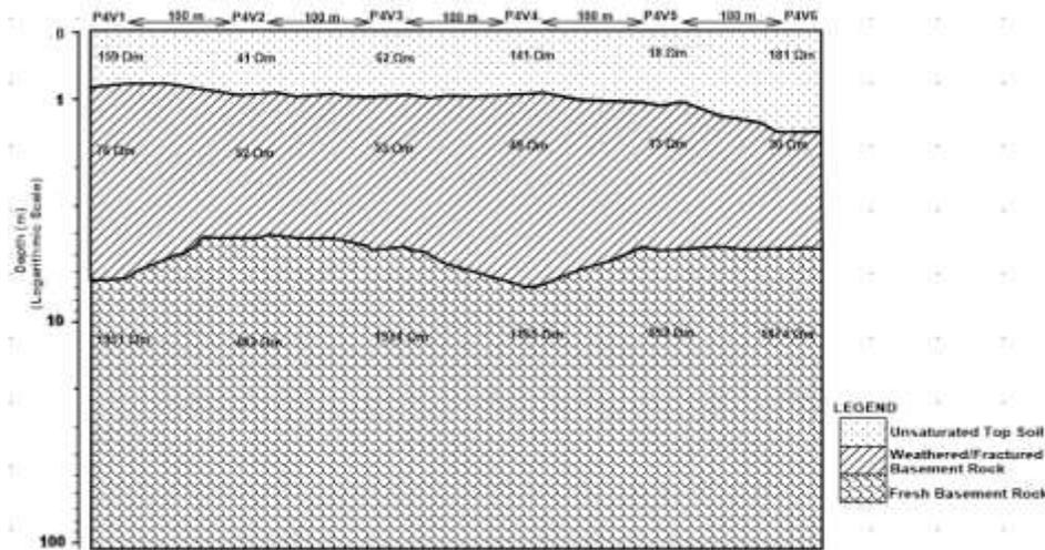
**Figure 11: Geoelectric/Geologic Section of Profile Four**
