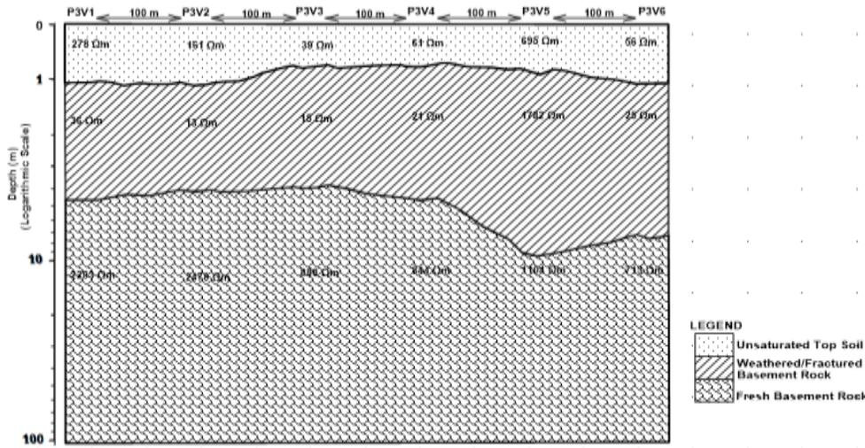
**Figure 10: Geoelectric/Geologic Section of Profile Three**
