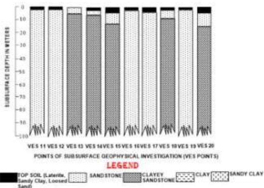
Figure 5: Geoelectric profiles for VES locations 11-20
