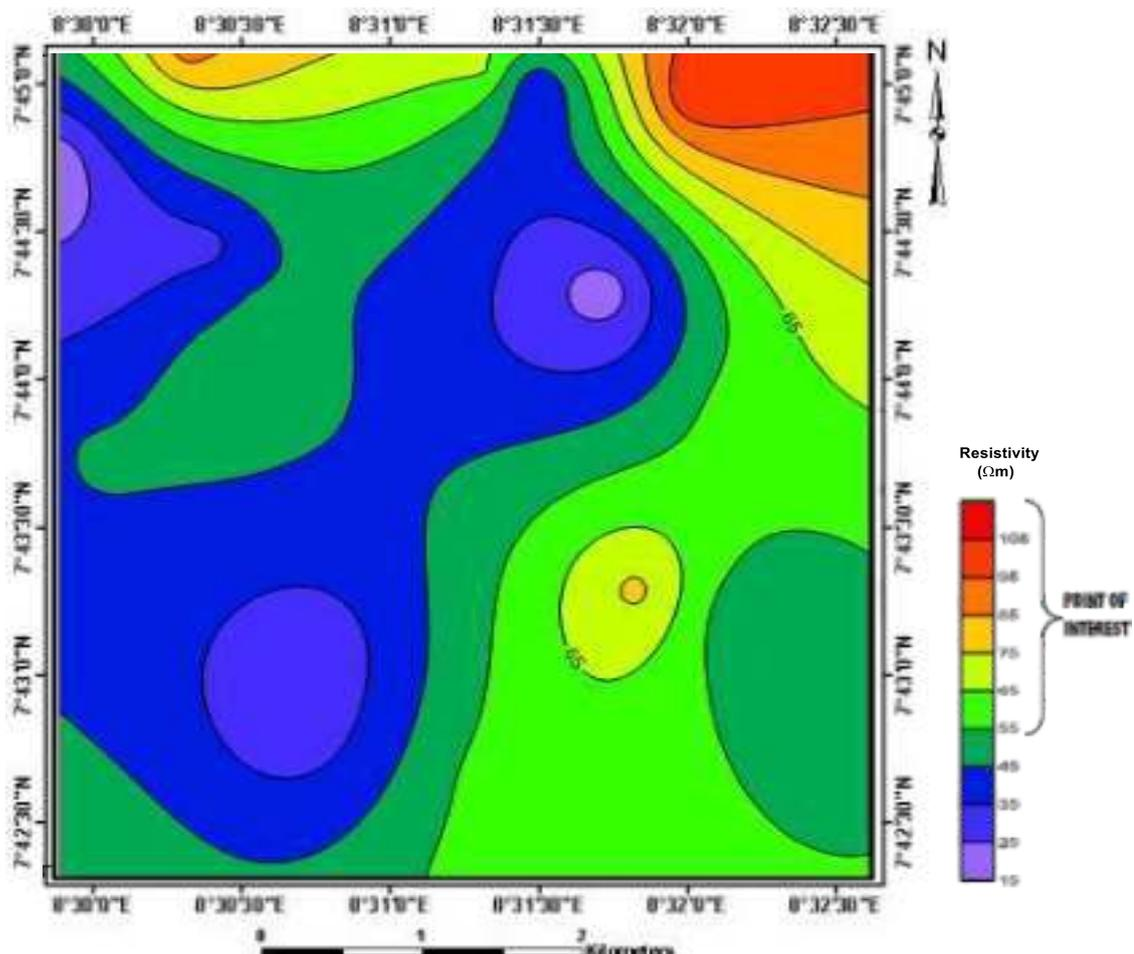
Figure 8: Isoresistivity contour at a depth of 20m
