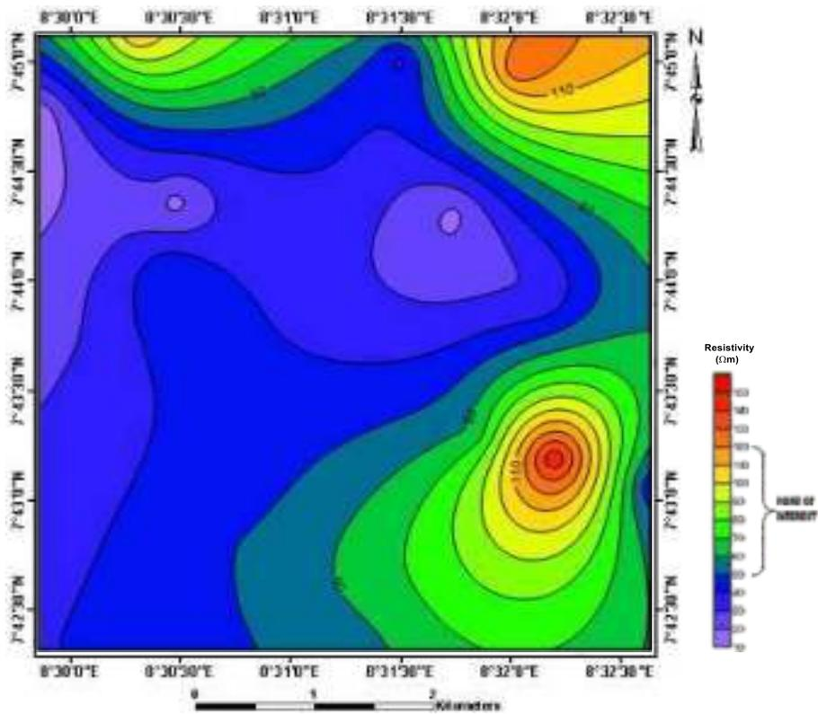
Figure 9: Iso-resistivity contour at a depth of 30m
