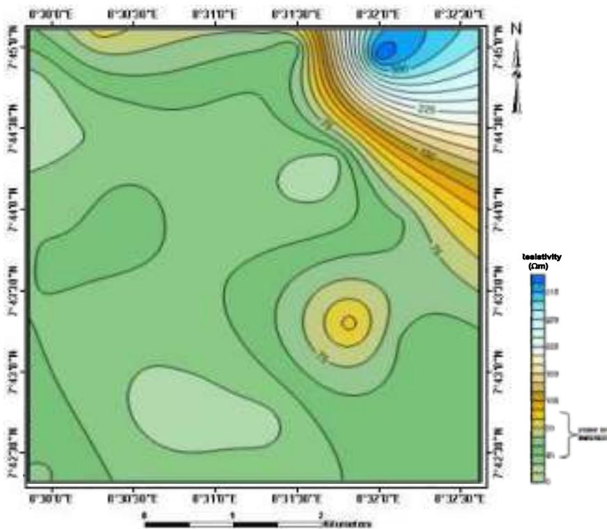
Figure 10: Iso-resistivity contour at a depth of 50
