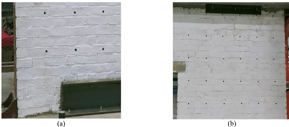
Figure 4. Failure modes of URM at different displacement loading. (a) Lateral crack at the base at 3mm (b) diagonal cracks at the edge of window opening towards the top at 4mm
