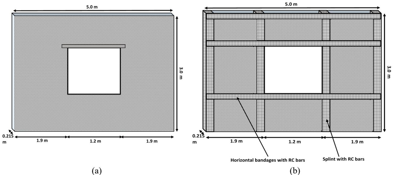
Figure 1. Schematic diagrams of the masonry wall: (a) unreinforced; (b) reinforced with splint and bandages.
