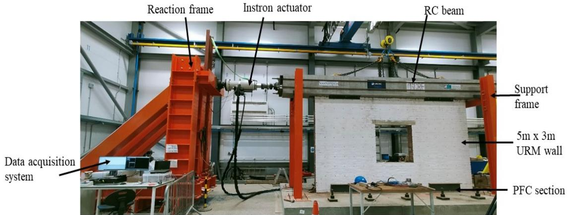
Figure 2: The experimental test setup
