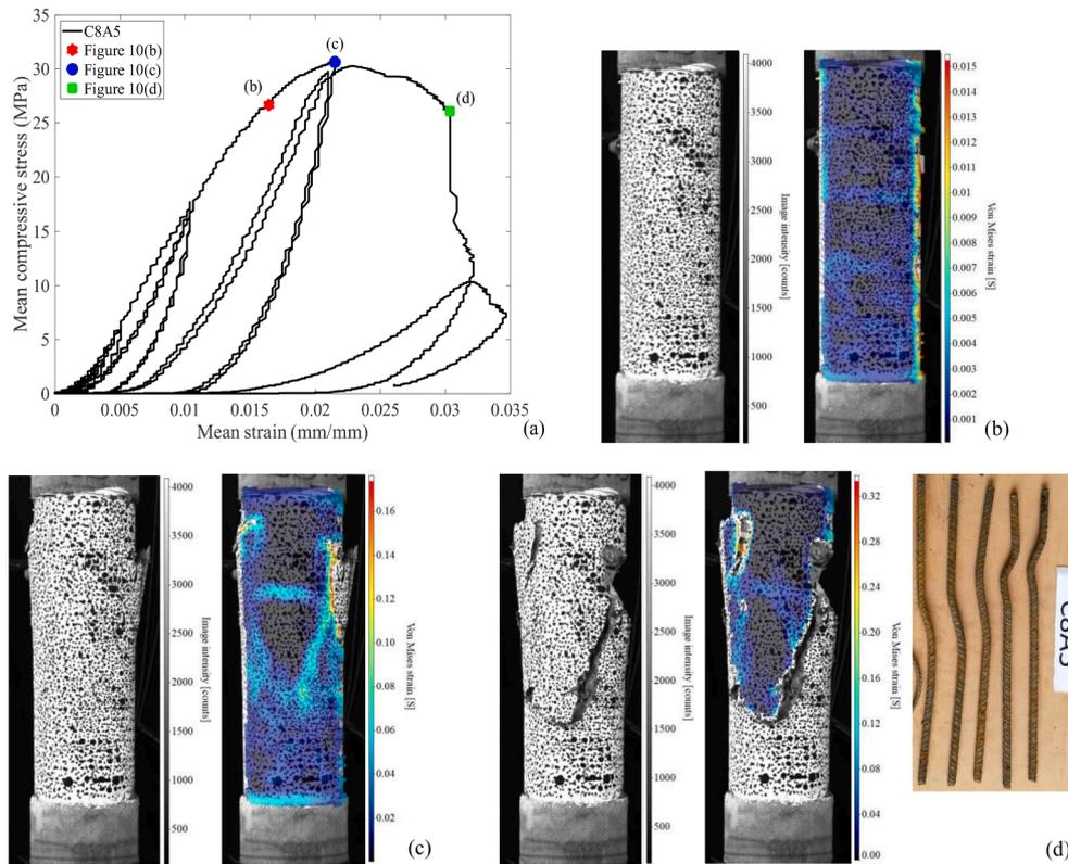
**Fig. 10.** Processed DIC images of circular column (a) stress–strain response showing location of processed images (b) at yield stress, (c) at ultimate stress and (d) between ultimate stress and collapse.
