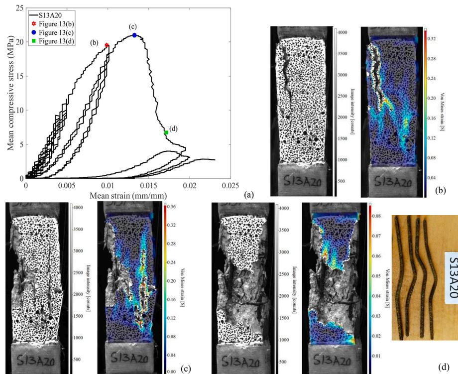
**Fig. 13.** Processed DIC images of square column (a) stress–strain response showing location of processed images (b) at yield stress, (c) at ultimate stress and (d) between ultimate stress and collapse with the buckling at the end of the test.
