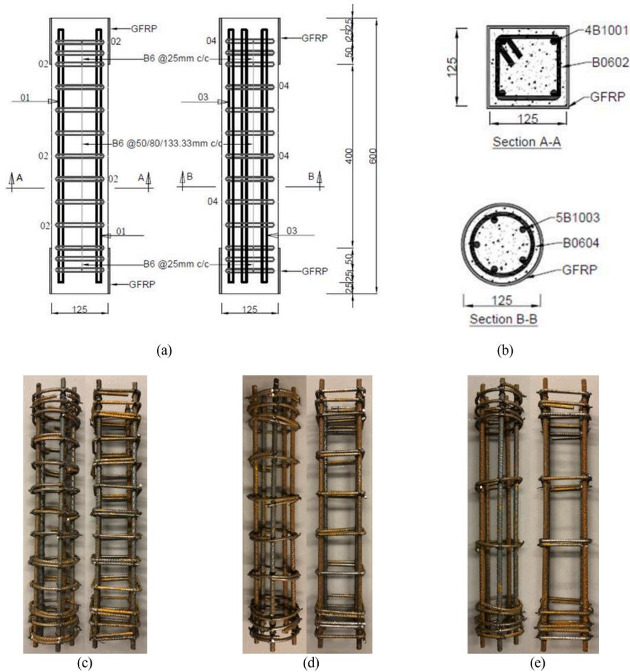
**Fig. 1.** RC columns details; (a) Elevation (b) Cross sections (b) High confined ( $L/D = 5$ ) reinforcement cages (c) Medium confined ( $L/D = 8$ ) reinforcement cages (d) Low confined ( $L/D = 13$ ) reinforcement cages.
