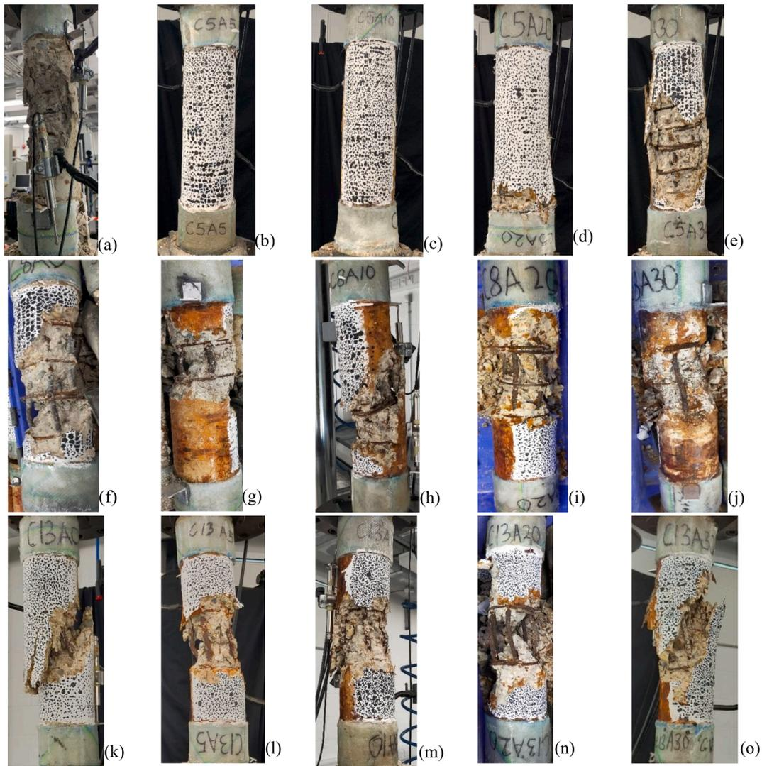
Fig. 9. Observed failure modes of circular columns with the different corrosion levels and confinement ratios; L/D = 5 (a - e), L/D = 8 (f - j) and L/D = 13 (k - o).
