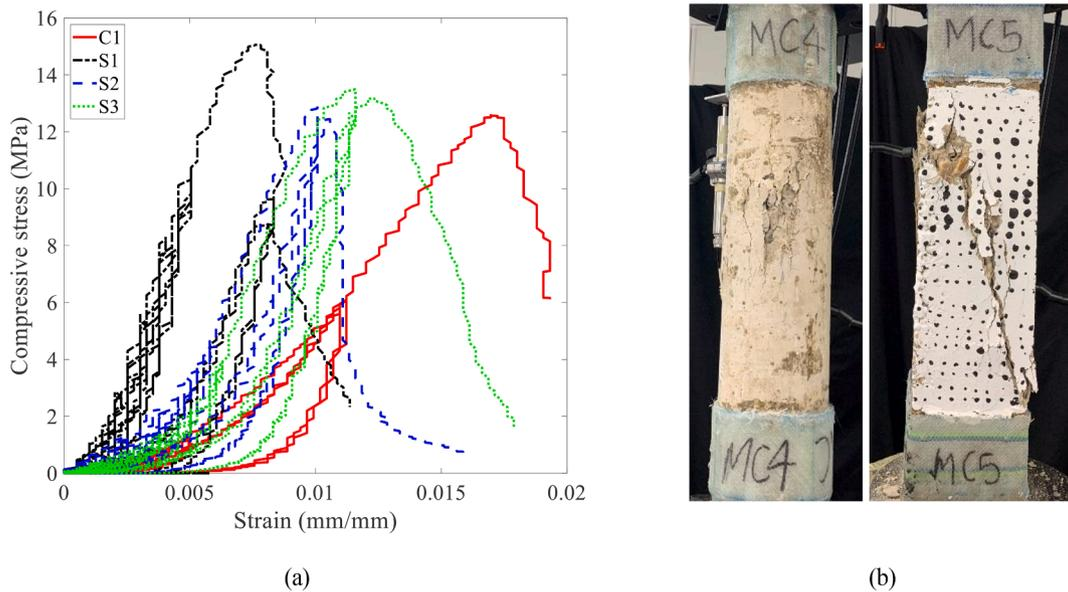
**Fig. 2.** Mass concrete behaviour (a) stress–strain response (b) observed failure after test.
