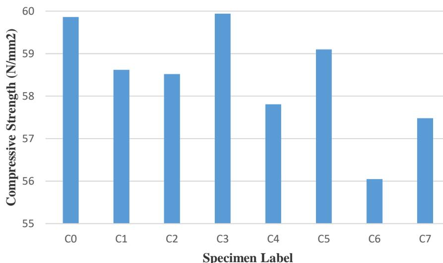
**Figure 3: compressive strength of HPCs at 28 days**
