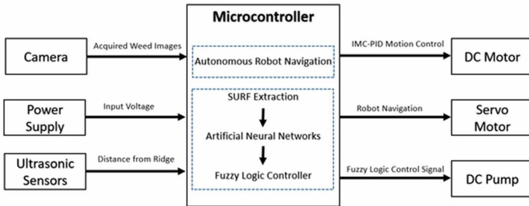
Figure 3. Circuit Diagram of Mobile Robot
