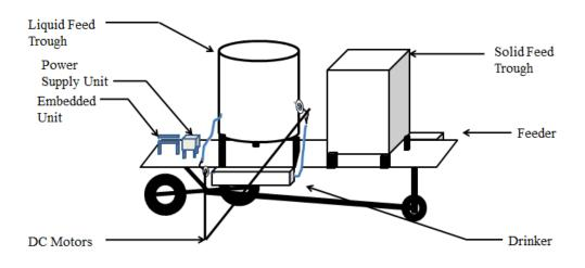
Figure 2: Overview of the mobile intelligent feed dispensing system
