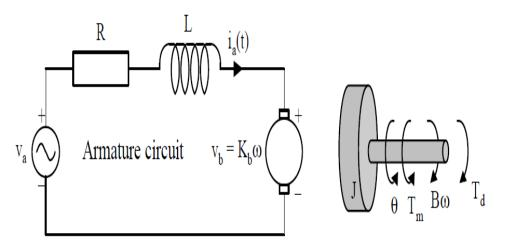
Figure 6: Model diagram of the solid feed trough of the dispenser
