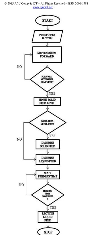
Figure 7: Mobile Intelligent Poultry Feed Dispensing System Flowchart
