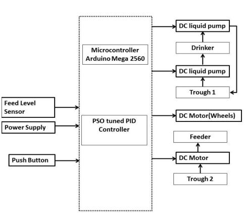
Figure 3: Block Diagram of the mobile intelligent poultry feed dispensing system
