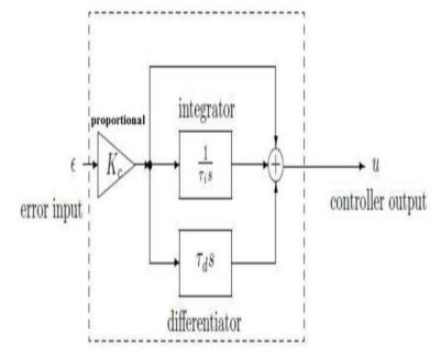
Figure 1: A PID Control System [27].
