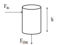
Figure 5: Model diagram of the liquid feed trough
