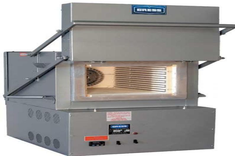
Figure 3.1: Cress single Chamber Annealing Furnace (SEDI, 2011).
