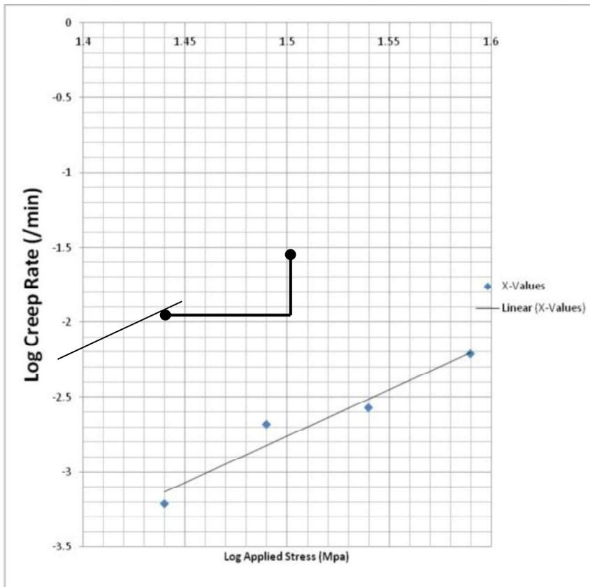
**Figure 8:** Log creep rate versus log applied stress
