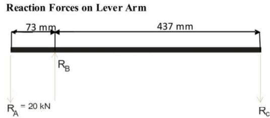
Figure 2: Free body diagram of reaction forces
