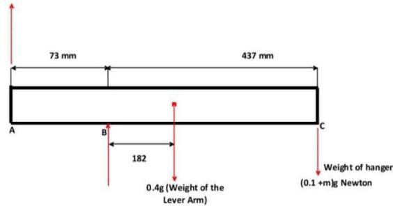
Figure 3: Forces acting on lever arm and specimen.
