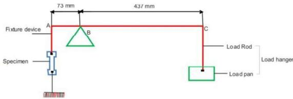
Figure 1: Systematic drawing of the creep testing mechanism
